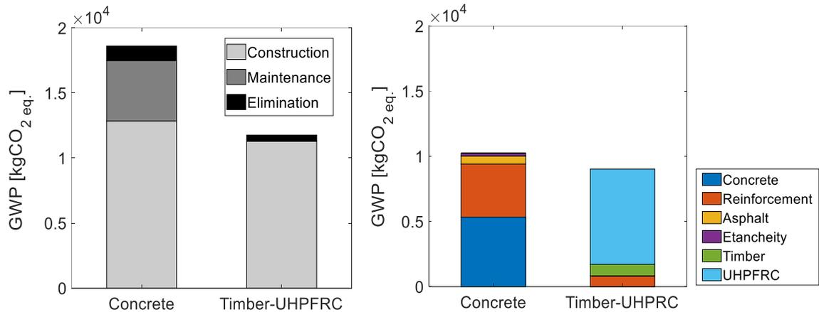
Figure 4 Environmental impact of bridge designs. A) Total impacts over the bridge service duration. B) impacts of the construction of the bridge superstructure.
