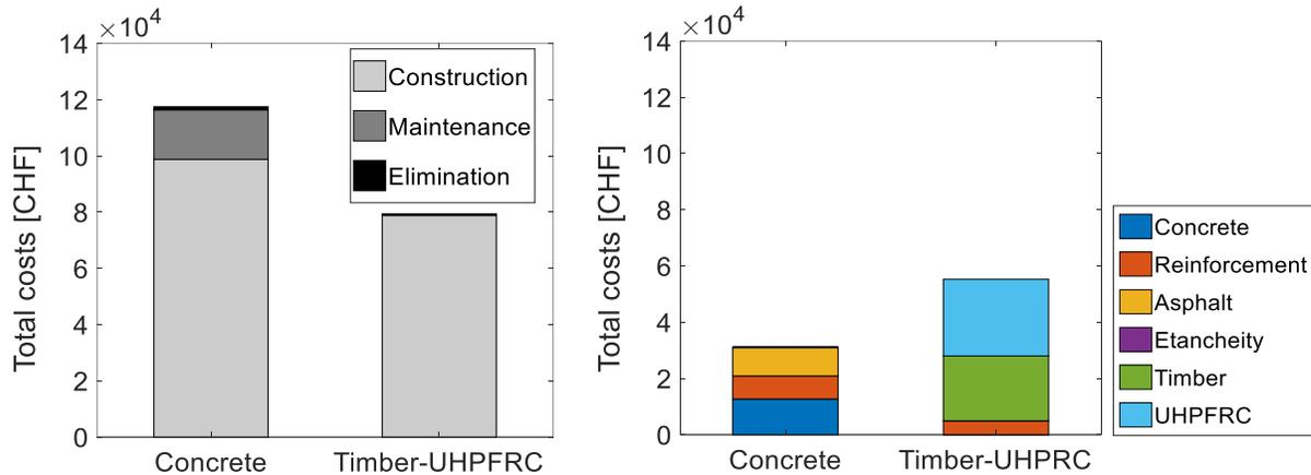
**Figure 5** Life-cycle costs of bridge designs. A) Total costs over the bridge service duration; B) Construction costs of the bridge superstructure.
