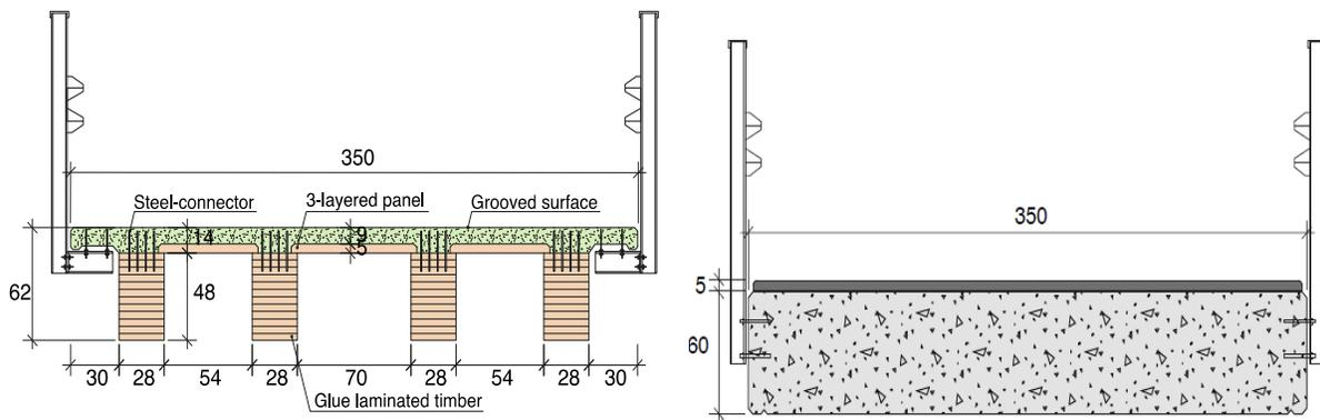
Figure 3 Alternatives: A) timber-UHPFRC; B) Reinforced-concrete bridge.
