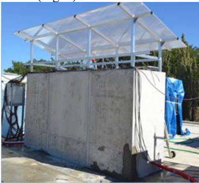
FIGURE 3: In-situ sample (100×200×400 cm 3 ) affected by swelling pathologies
