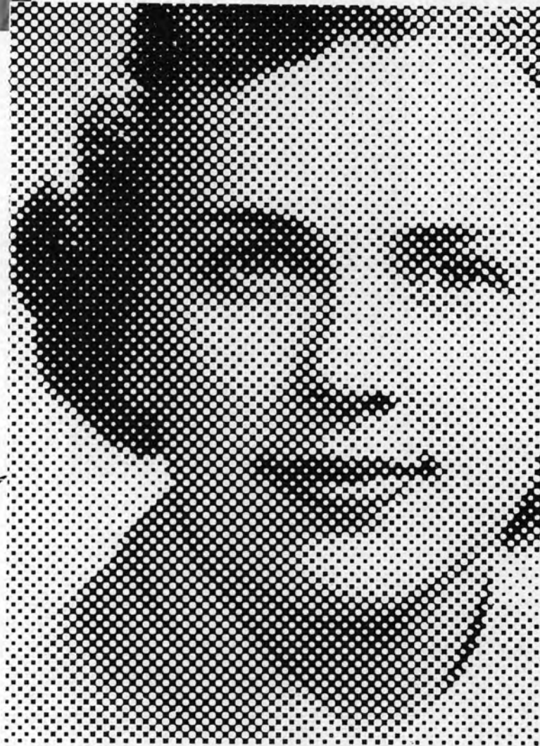
FIGURE 7.19. Enlargement of a halftone to show the dot pattern and screen effect produced by the halftone screen. Note that in the light areas of the skin the dots are small and widely separated, while in the dark areas of the hair the dots overlap. Notice how the eye blends the dots together into a recognizable image when this enlargement is viewed from a distance of six feet or more.
