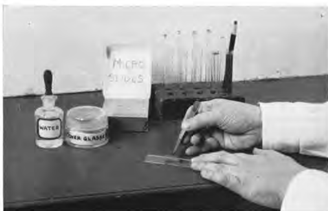
FIG. 13—Applying the coverglass, using forceps. DO NOT PRESS DOWN!
