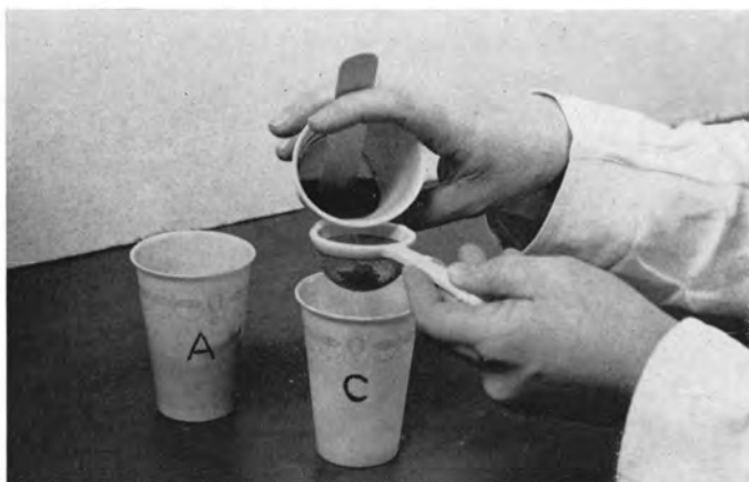
FIG. 5—The watery portion of container B is passed through the sieve into container C.
