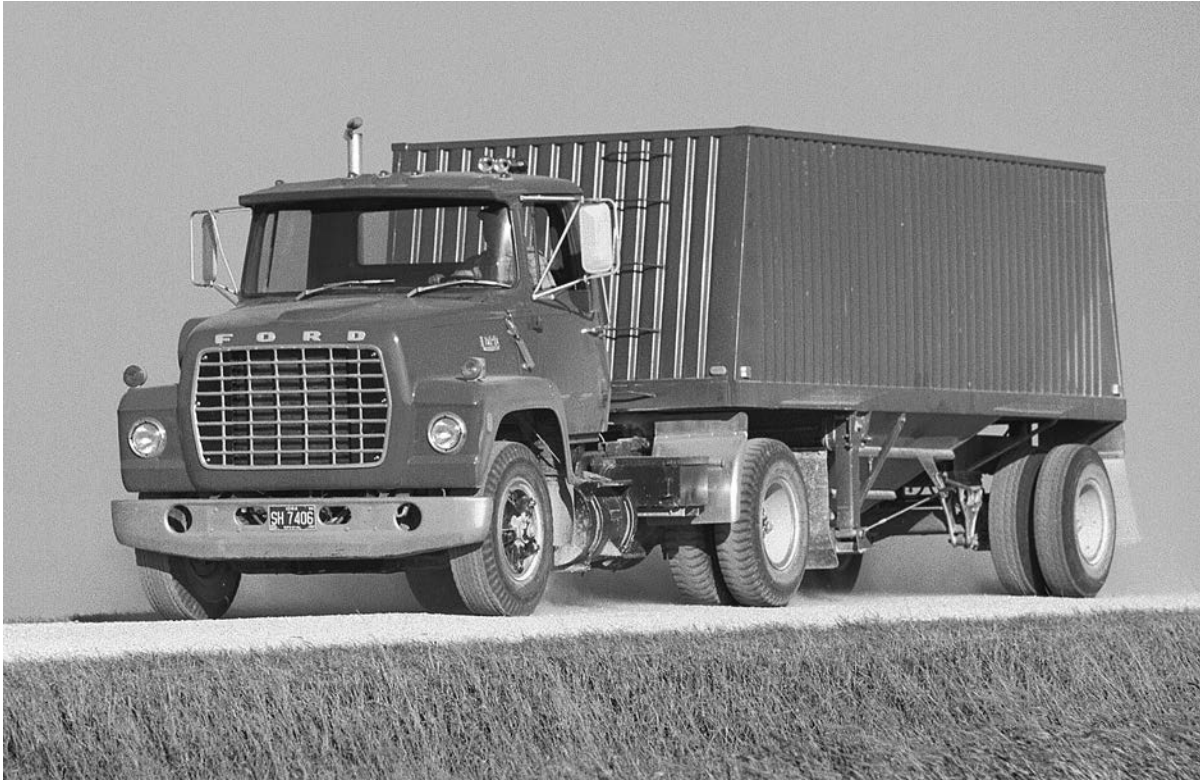
Mick and Sue Reigelsberger's grain-hauling tractor and semi-trailer. The tractor was white when Mick bought it used from the bottled water company in Humboldt. He then had it painted a fire engine red. The trailer has a capacity of 900 bushels of corn, but Iowa's Department of Transportation limits semi-trailer loads to about 830 bushels of corn. 1996.
