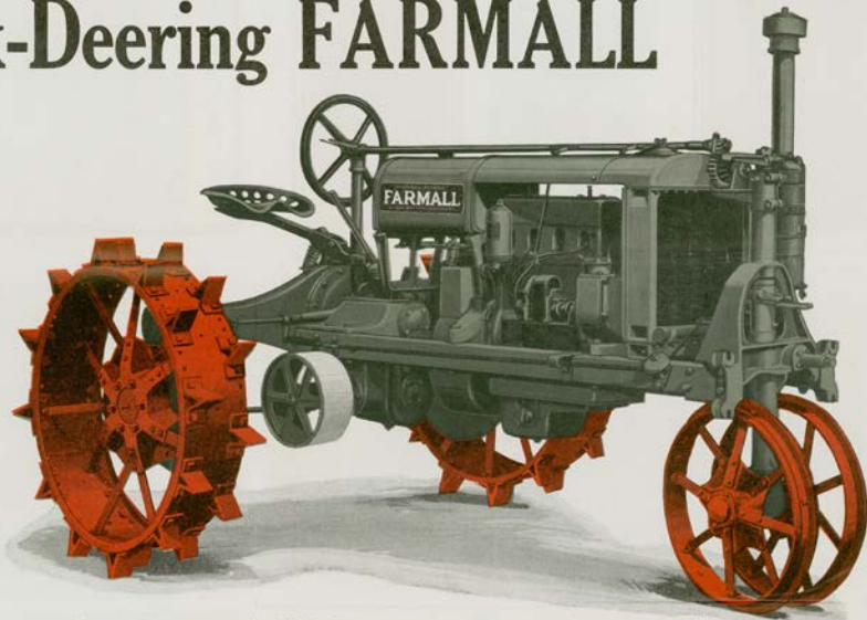
Illust. 1. This is the two-plow FARMALL—the tractor that is putting agriculture on a new and far more profitable basis. The wheels may be the 12 x 42-inch with spade lugs as shown, or 6 x 40-inch with angle lugs. Wheel equipment must be specified.
