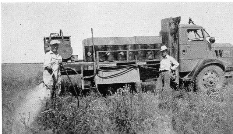
A new method of weed control was introduced in 1927—use of sodium chlorate. This large power sprayer, county-owned, is typical of the type in service to treat European bindweed and other perennial weeds with the chemical.—CHAPTER 8, WEEDS THAT CHALLENGE IOWA CROPS.
