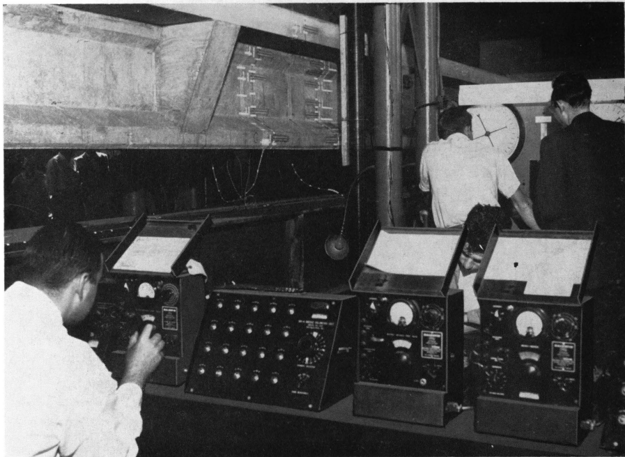
In this research project the civil engineer is testing a prestressed concrete bridge beam in a testing machine capable of applying a load of 400,000 pounds. The electrical equipment in the foreground is being used to measure the effects of loads applied with the testing machine.
