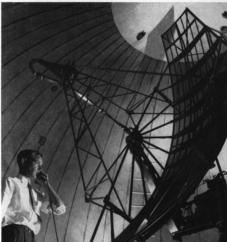
This electrical engineer is receiving data on tests of radar height-finder. Radar's energy is concentrated in a narrow beam like that of a search-light and is powerful enough to light fluorescent lamps one hundred feet away. (Courtesy General Electric Co.)
