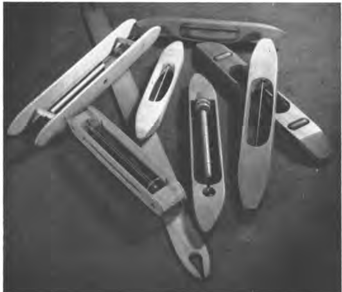
Fig. 2.9—A few of the many types and sizes of shuttles. At the extreme right, rollers in the bottom of the shuttle eliminate friction. The flat stick accommodates wefts too bulky or wiry to be wound in the usual manner. The shuttle in the center foreground uses a wooden bobbin. With the others, paper quills or spool-like bobbins of wood or plastic are used.
