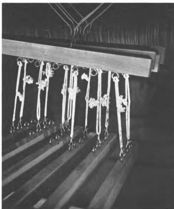
Fig. 6.12—Standard tie-up uses all six treadles. Here the tabby treadles are at the right, tied to Lams 1 and 3, 2 and 4, the four twill treadles at the left. Other arrangements are possible to suit comfort of weaver.
