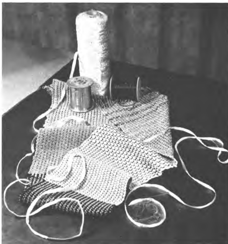
Fig. 4.8—A sample warp removed from the loom. Rayon roving weft or filler, black cord, heavy linen, and chenille used in the warp.
