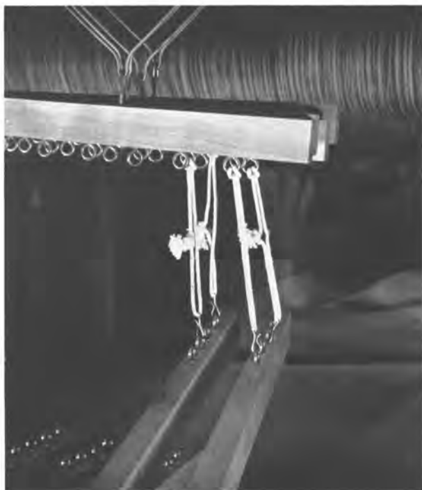
Fig. 6.10—Treadle tie-up for plain or tabby weave. Treadles at lower front are attached by cords to the lams (wooden bars running cross-wise), and these in turn are hooked to metal rods fastened to the harnesses. Right treadle is hooked to Lams 1 and 3; left treadle to Lams 2 and 4.
