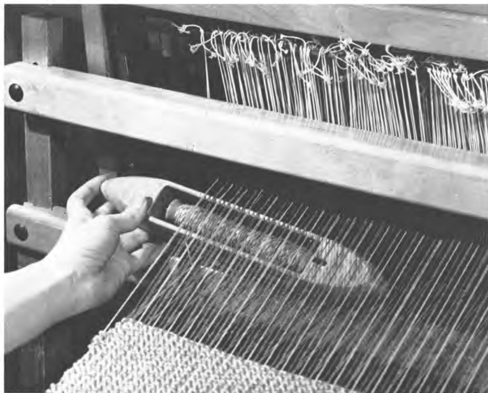
Fig. 7.4—Throwing the shuttle. Holding the shuttle as illustrated, it is pointed slightly toward the beater and thrown across close to the beater. Properly thrown in a good shed, the shuttle moves across smoothly and quickly.
