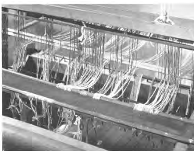
Fig. 6.6—Reed is threaded according to a planned spacing. Note the reed is in position across the front, resting on the front-to-back bars. After threading is completed, reed will be placed in position in the beater. Warp is for a bamboo screen.
