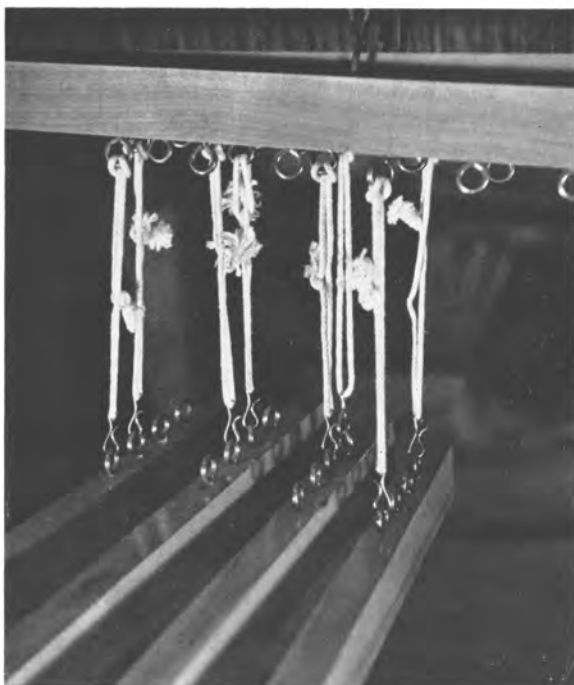
Fig. 6.11—Tie-up for simple twill. Note the 1 and 2, 2 and 3, 3 and 4, 1 and 4 combinations. A twill results when treadled either from right to left, or left to right.
