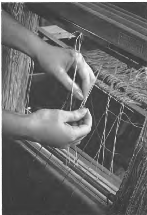
Fig. 6.5—Threading the heddles. Starting at the back harness, the yarn that was held between the thumb and first finger has been threaded through the heddle on Harness 4; yarn held between first and middle finger, through heddle on Harness 3; third yarn in the left hand is being threaded through heddle on Harness 2; and the fourth warp end farthest to the left will be threaded through heddle on Harness 1.
