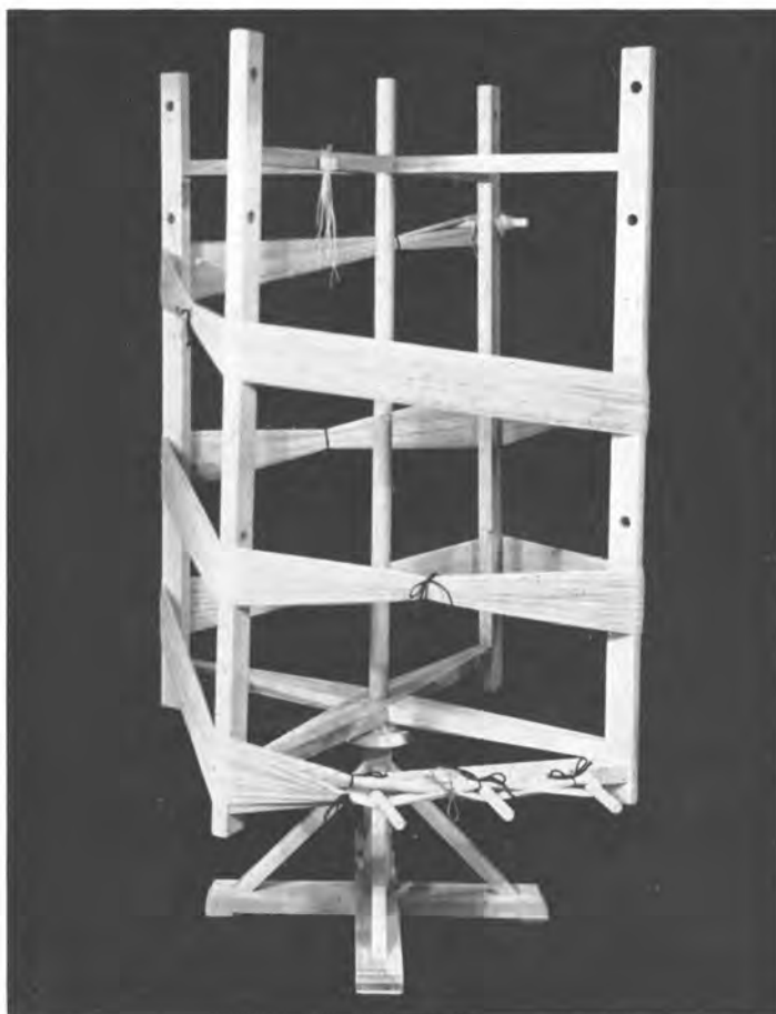
Fig. 5.4—Warping reel with completed warp, showing how it was looped around the starting peg, the cross in place at the bottom, all ties in place, the whole warp ready to be removed.
