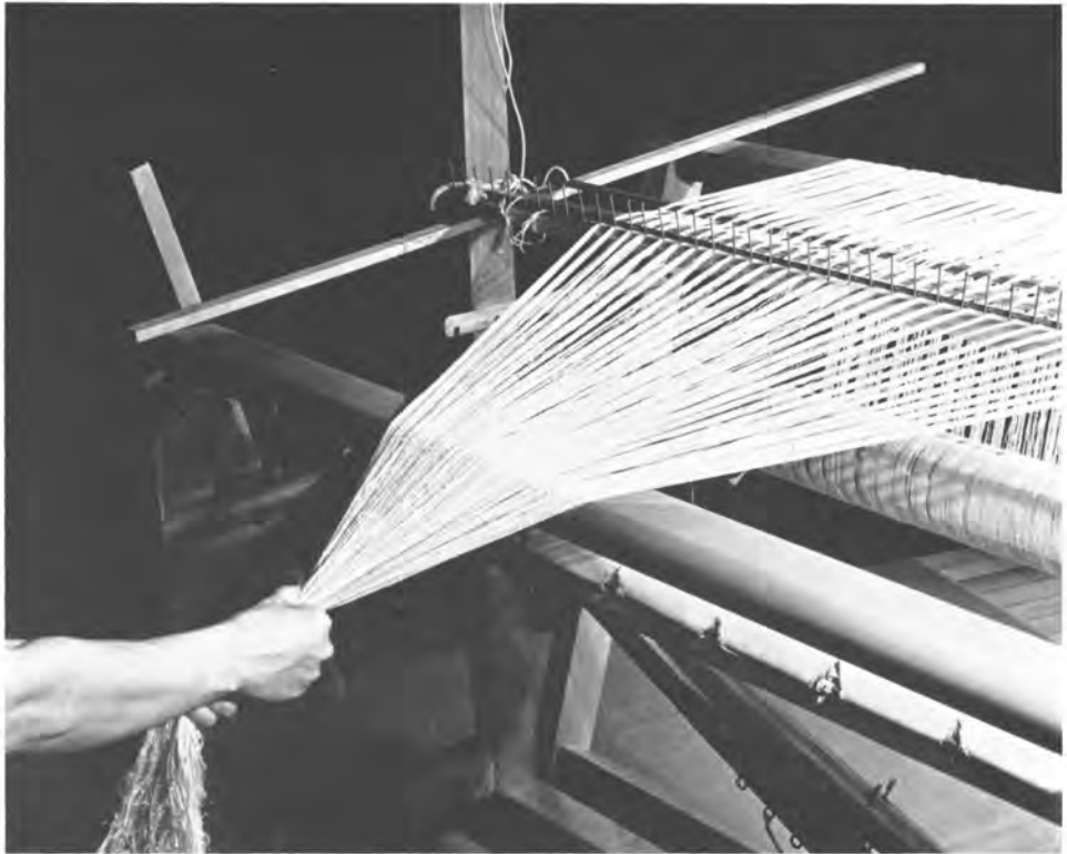
Fig. 6.2—Warp gathered together and held down firmly over the breast beam. Cord and rod at the spreader hold warp yarns in place. Spreader and lease sticks are supported by slats which reach from front to back and are tied to the loom uprights. Harnesses have been removed.
