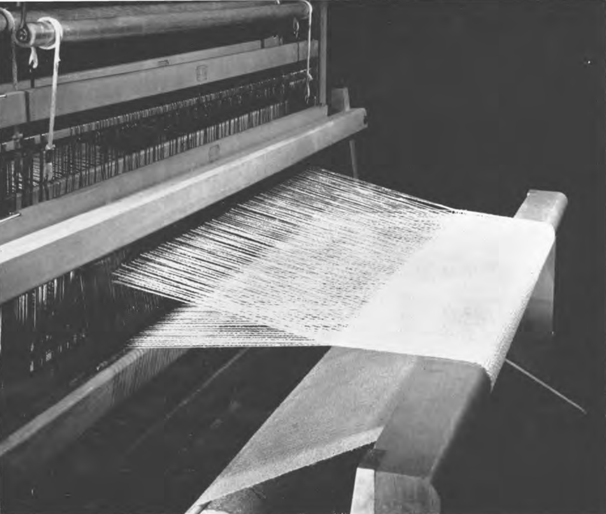
Fig. 7.1—A clean shed. Lower warp yarns lie in a level plane along base of the reed, forming a smooth path for the shuttle to move across.
