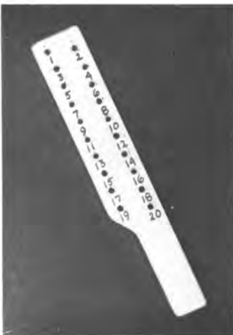
Fig. 2.7—The paddle used when winding warps of four or more yarns. Numbered holes show the order of threading the warp ends.
