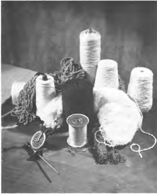
Fig. 2.4—Yarns packaged on tubes, spools, cones, and in skeins. Note skein of chenille in background and white loop mohair at front. Linen tow yarn gives a dull texture to the tall spool, while the smooth white cone at left front is a mercerized cotton.
