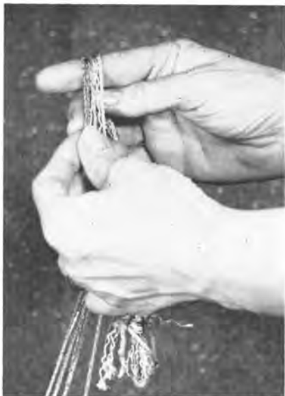
Fig. 4.4—Finding a suitable warp unit, by arranging yarns in different sequences until the most satisfactory one is found.
