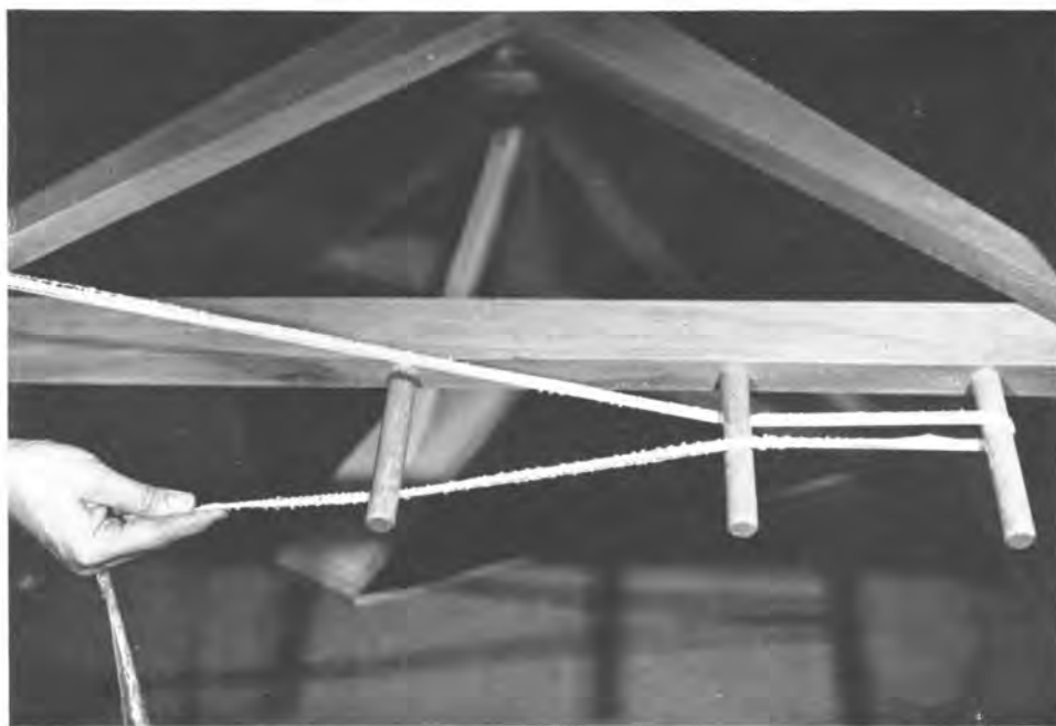
Fig. 5.3—Yarns in the unit are wound together around the three pegs at lower end to form the cross.
