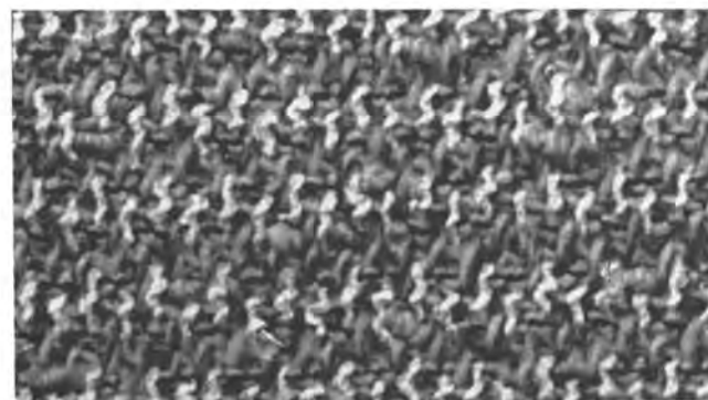
Fig. 4.25E—Drapery with a rich, textured surface. Warp is a 2-ply wool of gray and white alternated with white rayon ratiné; filler, a novelty yarn of wool in black, natural, and flakes of yellow, twisted together. Weave is broken twill.
