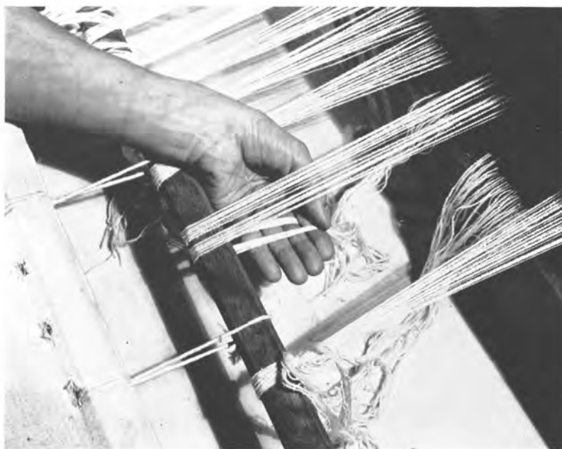
Fig. 6.7—Tying warp to cloth apron. In the first step, a unit of yarns coming through the reed is brought over the warp stick and divided into two sections. Warp stick has been tied to cloth apron at regularly spaced intervals.
