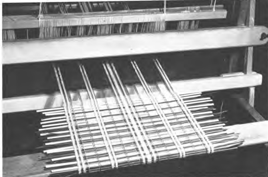
Fig. 4.14—Design for place mats showing open spacing in the reed. Note the harnesses here consist of parallel bars of wood to hold cord heddles in place. Threading is twill, weave is tabby. Warp is brown linen, chartreuse mercerized cotton, and white chenille; filler is natural bamboo and brown Nigerian reed. (Student project at the State University of Iowa.)
