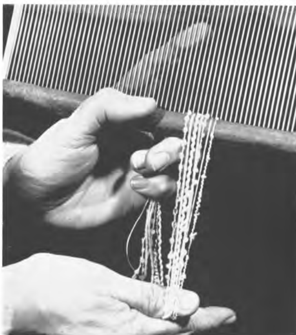
Fig. 4.5—To determine the spacing before winding the warp, the yarns selected are threaded through the reed. If they seem too close or too far apart a different reed may be selected or the yarns may be regrouped.
