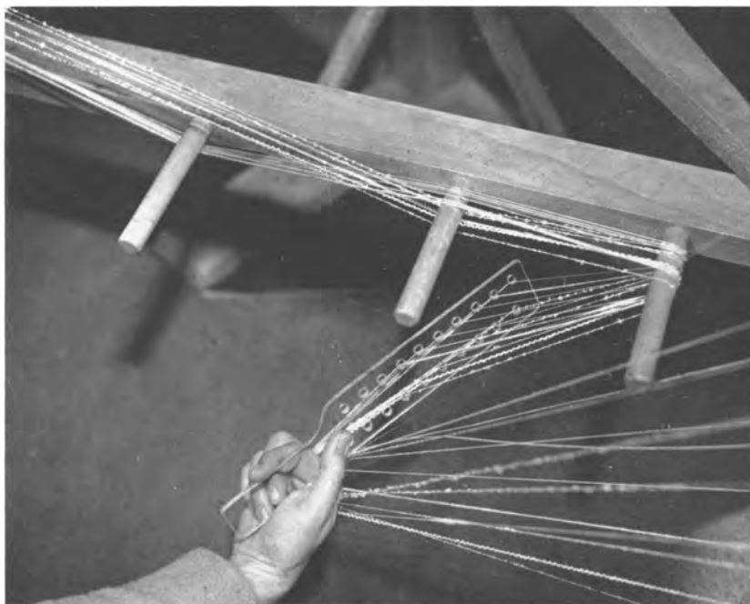
Fig. 5.10—Paddle passed around the end peg, ready to make the return cross. Note the wrist is turned to the right with Number 1 hole on top.
