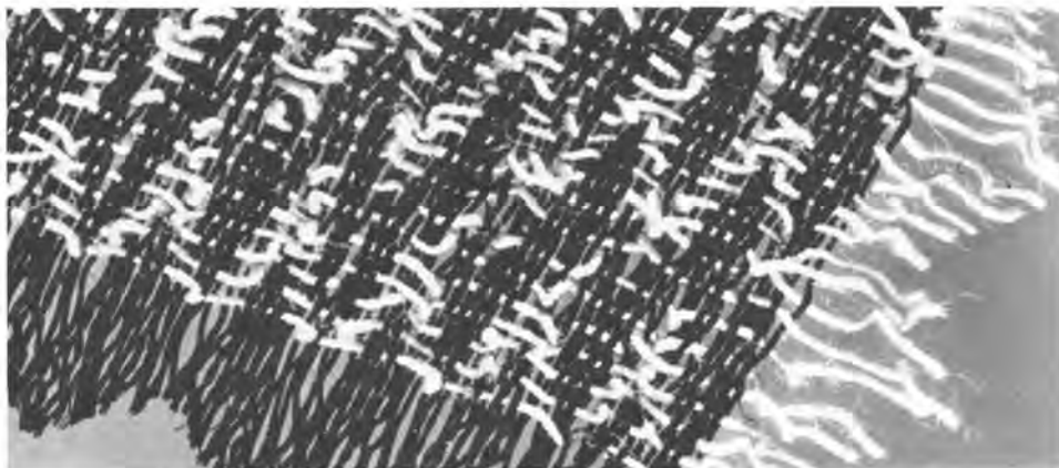
Fig. 3.6—Fabrics of Estron (acetate) plus other materials such as silk, wool, or cotton can be dyed in two-tone effects by the process “cross dyeing.” (Courtesy Tennessee Eastman Company.) Acetate resists the dyes that color the other fibers and they, in turn, resist the acetate dyes.
