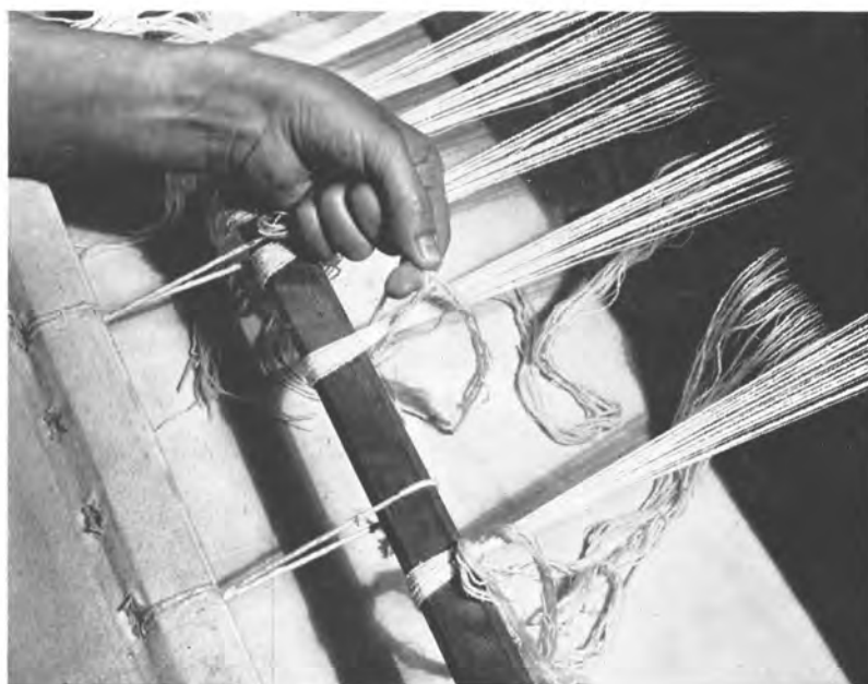
Fig. 6.8—Second step is to tie the temporary knot. Divided sections are brought around outside and over whole group and tied in a simple knot.
