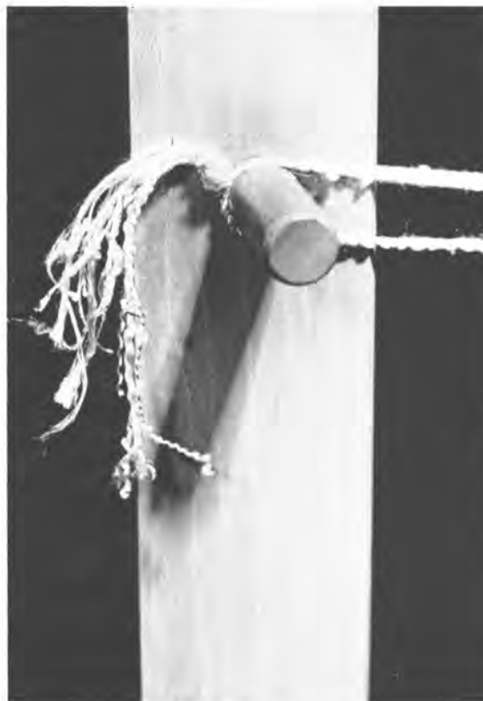
Fig. 5.2—Ends of the yarns in the warp unit have been tied together and slipped over the starting peg.
