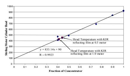
Assumption: The reduction in solar radiation, as the parabolic mirror is moved from 0.5 meters to 1.0 meters from the reflecting surface, is due to the divergence of the energy beam in a conical pattern. The diverging angle of the conical pattern may be determined by calculating the increased area necessary to capture the same amount of energy, see Figure A2. The diverging beam forms an annulus at the entrance plane of the parabolic reflector:
