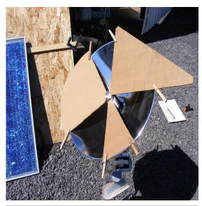
FIGURE 2. STIRLING CONCENTRATOR, 60% BLOCKED
