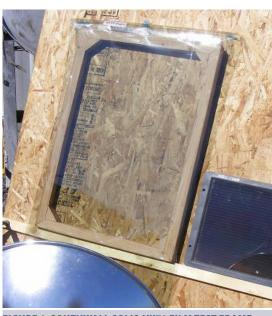
FIGURE 4. SOUTHWALL SOLIS-VK70 FILM TEST FRAME, NEXT TO PV PANEL
