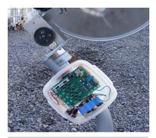
FIGURE 3. STIRLING ENGINE TRACKING DEVICE.
