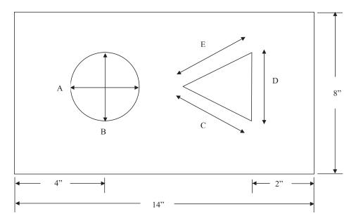
Each mounting plate consisted of one four-inch circle and one four-inch equilateral triangle. Each letter (A-E) located by the arrow represents the diameter or side from where the measurements listed in Table 1 were taken.
