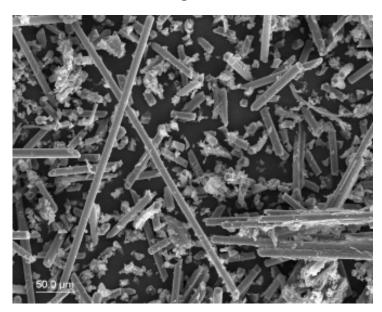
A sample of the recycled fiberglass composite powder was examined under an electron microscope. The A-arrows represent examples of the long and short rods of the fiberglass. Three granular shaped examples of the epoxy resin are represented by the B-arrows. The C-arrows show the interface bond separation between the fiberglass rods and the epoxy resin (photo furnished by Central Michigan University's Electron Microscopy Facility).
