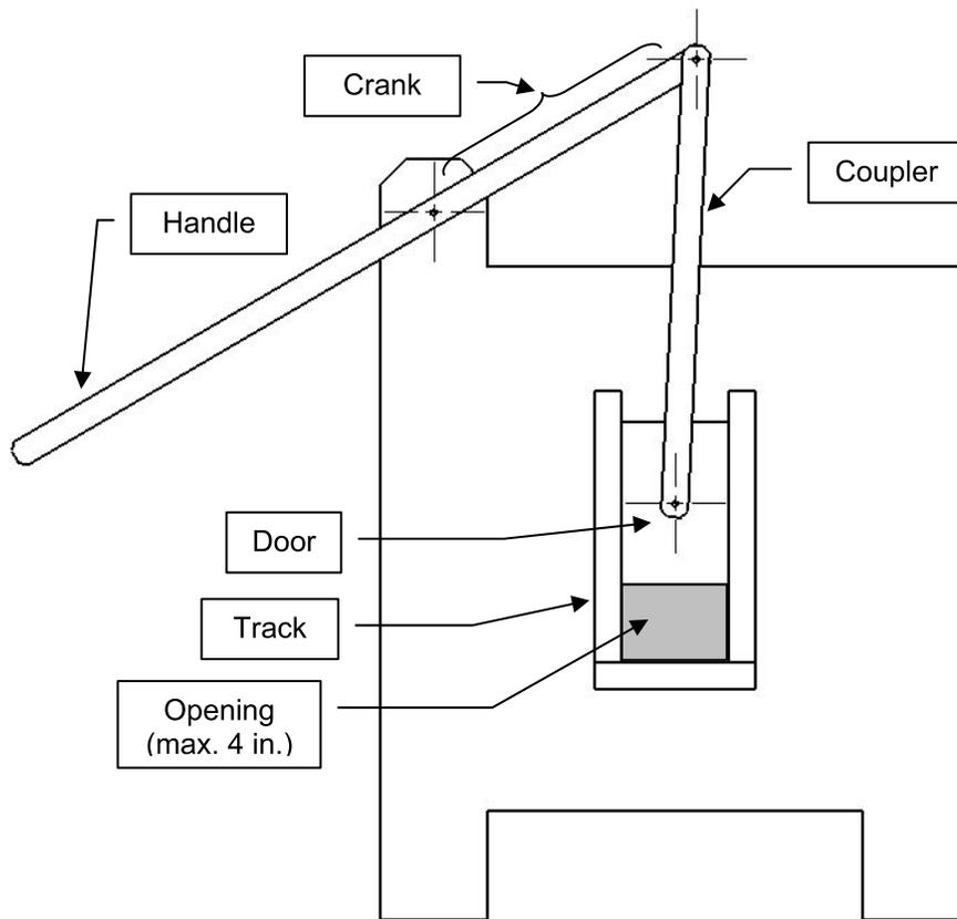
Figure 4. Schematic of oven with door opening mechanism
