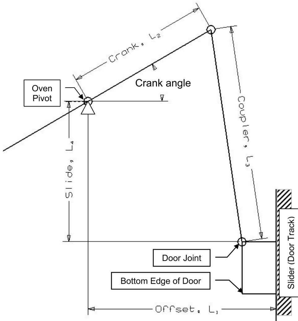
Figure 5. Kinematic diagram of oven door mechanism
