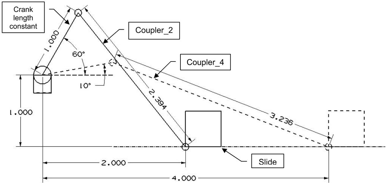
Figure 1. Schematic of crank slider mechanism
