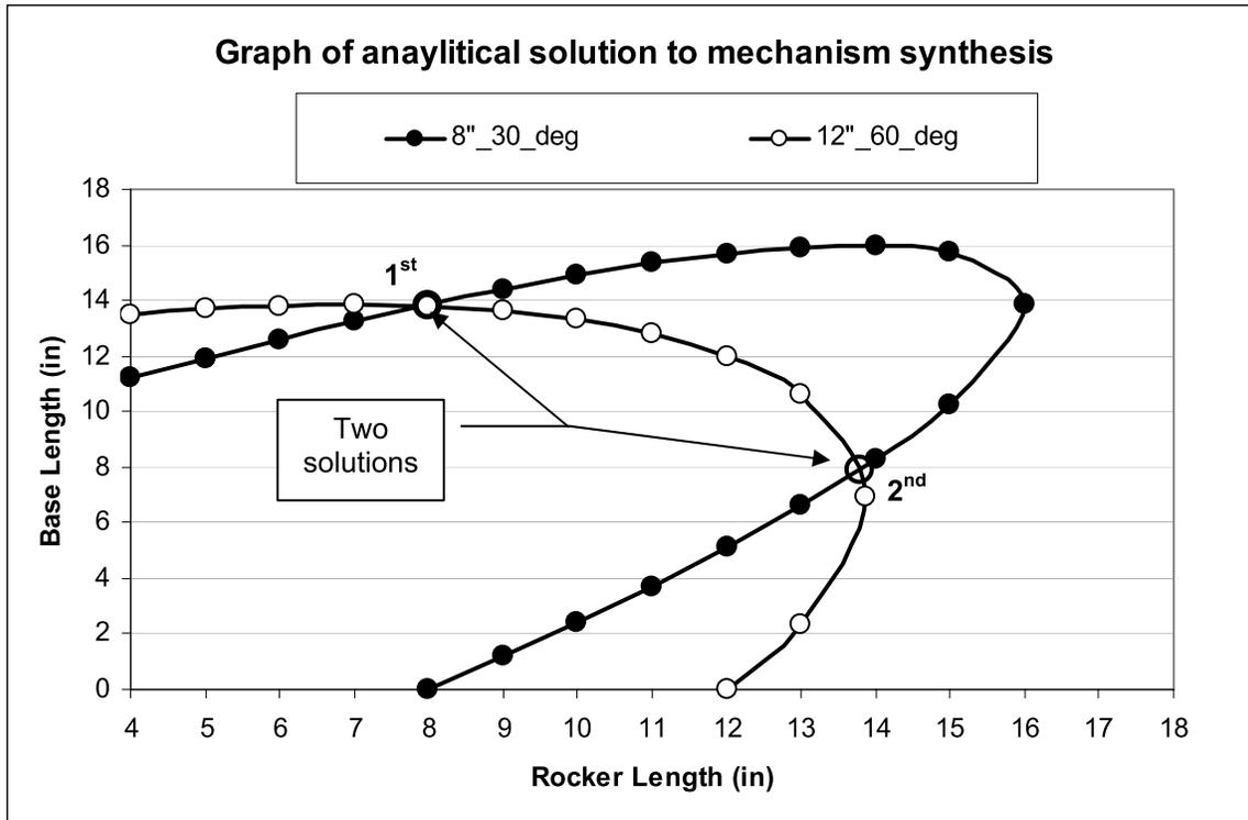
Figure 14. Graph illustrates two solutions possible for the tilt mechanism design
