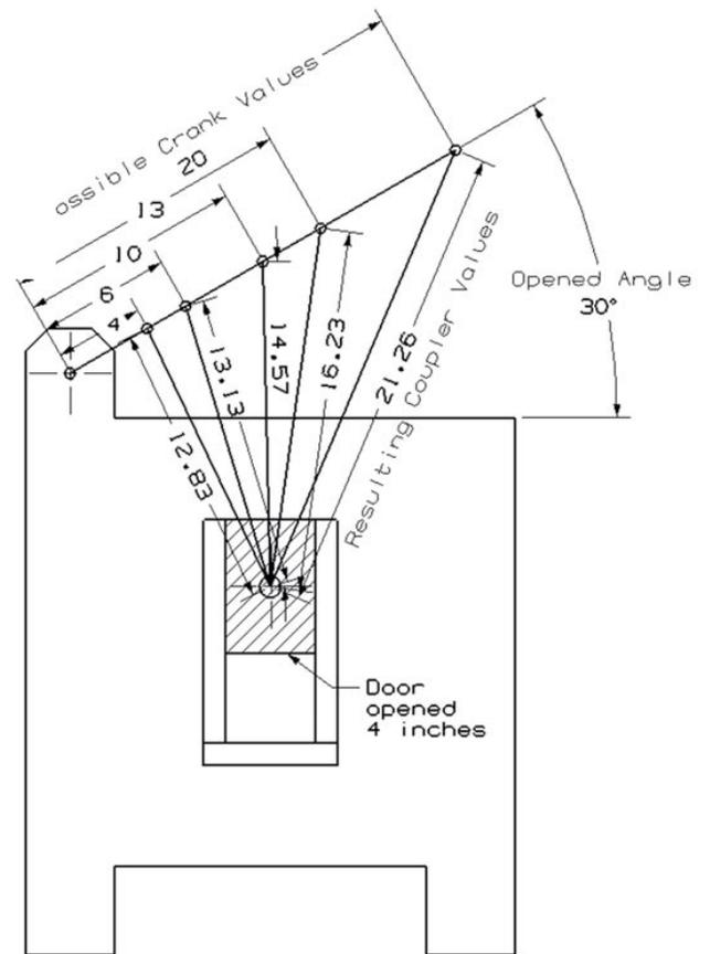
Figure 7. Representative pairs of crank and couplers satisfying the opened constraint
