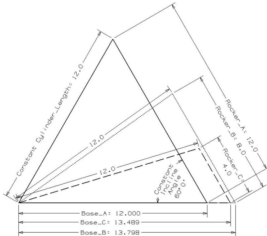
Figure 12. Overlay technique used to satisfy the extended cylinder constraint
