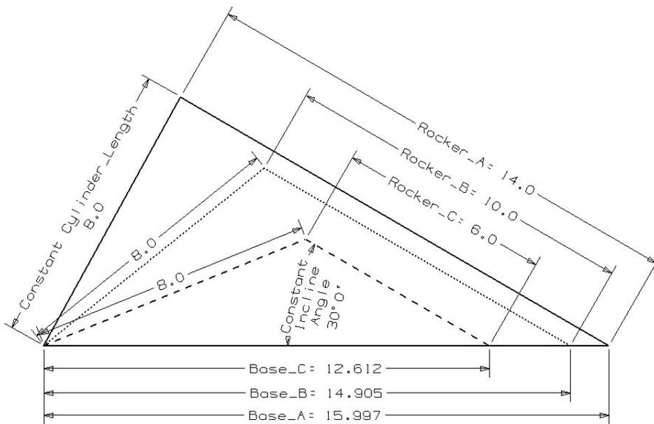
Figure 11. Overlay technique used to satisfy the retracted cylinder constraint
