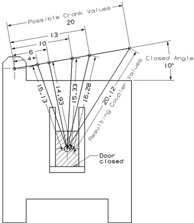
Figure 6. Representative pairs of crank and couplers satisfying the closed constraint
