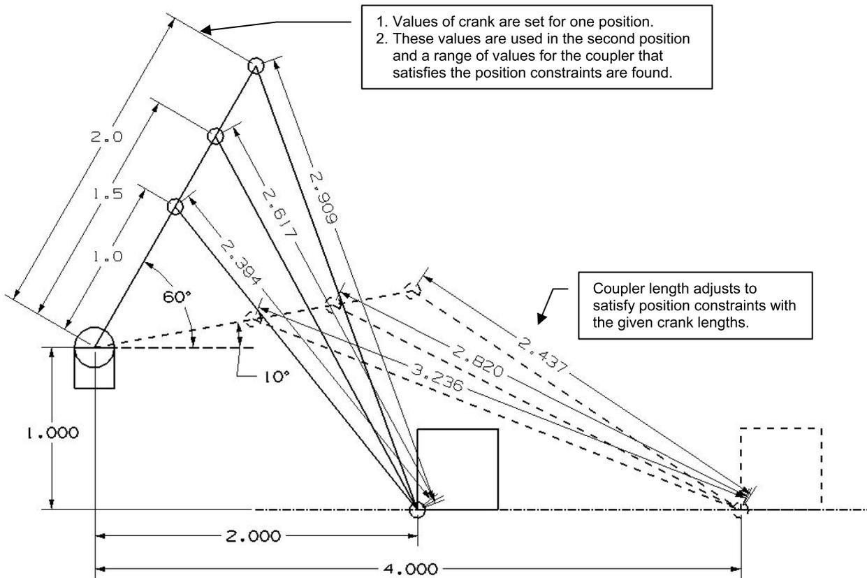
Figure 2. Overlay technique used to determine crank-coupler pair that solves design problem
