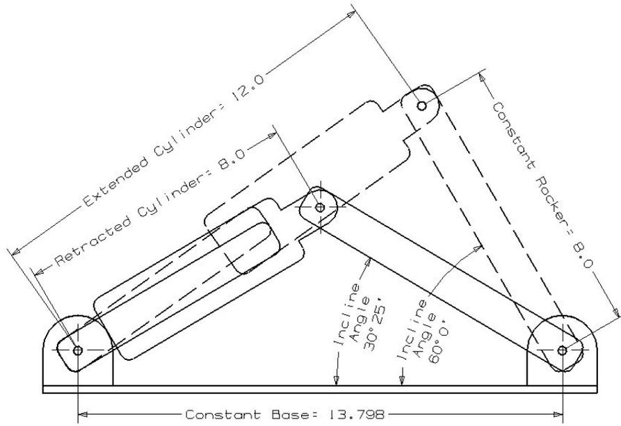
Figure 15. Overlay of 1st solution shown in Figure 14
