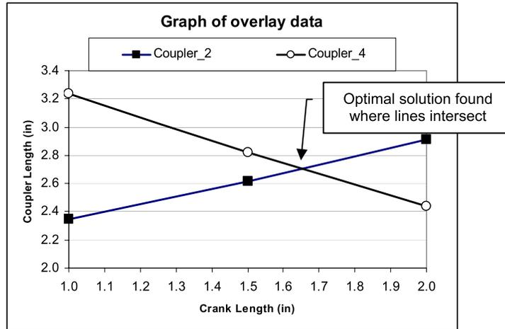
Figure 3. Optimal solution can be found by graphing results of overlay technique
