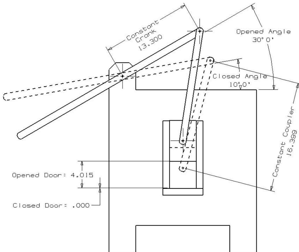
Figure 9. Overlay of the optimized door opening mechanism at the closed and fully opened positions
