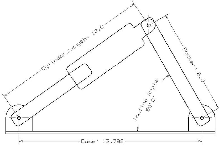
Figure 10. Schematic of Cylinder Incline Mechanism
