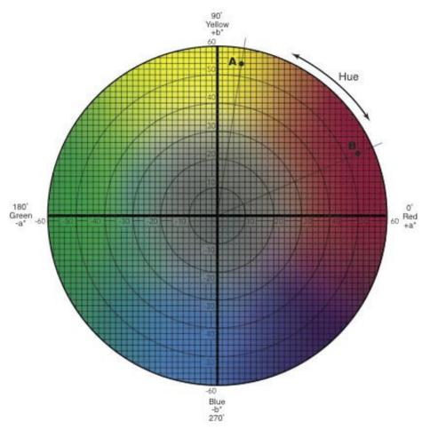
Figure 3: Schematic Diagram of CIE L\* a\* b\* Color Model (Courtesy of X-Rite)
