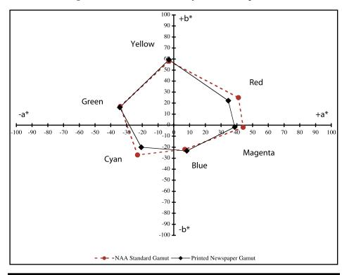
ments in newspaper color printing have made it possible for newspapers to offer quality color printed advertisements. The most difficult task of this experiment has been the ability to collect reliable measurements from the preprinted samples. The density level in the newsprint varies frequently due to several technical and non-technical factors. This made it impossible to obtain accurate data values that match with NAA standards.
