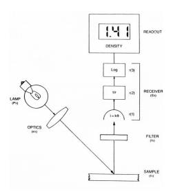
Figure 2: Schematic of a Densitometer (Courtesy of GCA)
