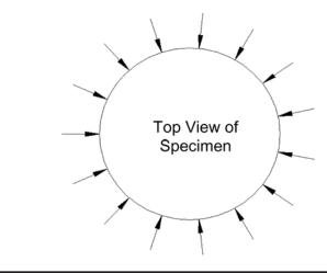
Figure 5. Axial measurement planes. This illustration designates the three axial measurement planes which will be sampled for each specimen. As shown, three axial planes (fifteen points each) will be sampled in the following locations in inches relative to the top of the specimens.
