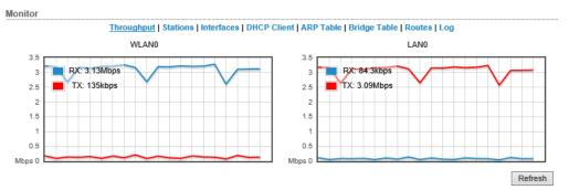
Fig. 7 Receive and transmit data rates for streaming video from four webcams
