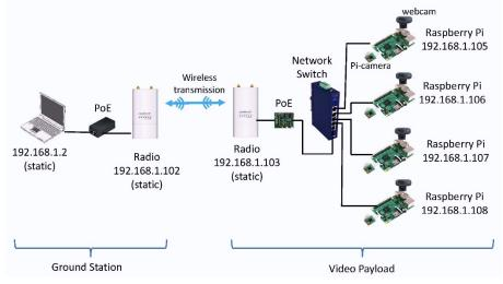
Fig. 1 Functional block diagram of the multi-streaming video payload.
