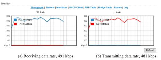
Fig. 6 Receive and transmit data rates for streaming video from four Pi-cameras
