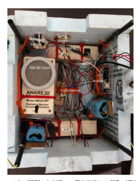
Fig. 1. The instrumentation of UMM payload #1flown on Flight #1 (19 August 2017) and Flight #5 (21 August 2017). It contains two RM-60 GMs for the detection of omnidirectional cosmic rays and two stacked RM-80 GMs for the detection of vertical cosmic ray coincidence counts. Temperature and pressure sensors are also included.
