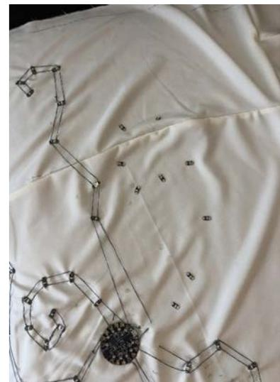
*Figure 2 Process of sewing the circuit of individual LEDs inside the dress*
