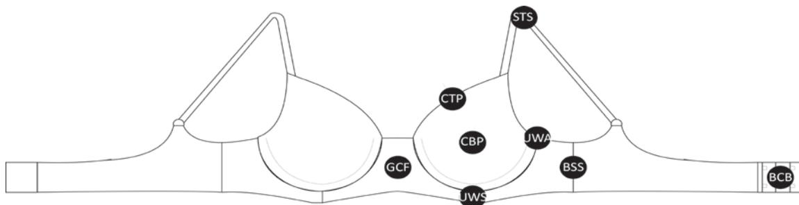
Figure 1. Pressure measurement locations on a bra prototype
