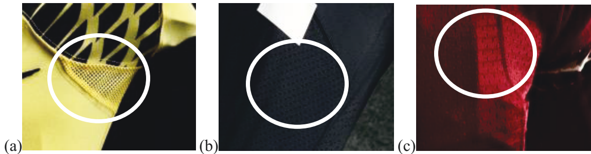
Figure 1. Three types of vent designs in athletic football uniforms: (a) chain-maille mesh, (b) laser perforated mesh, and (c) traditional mesh
