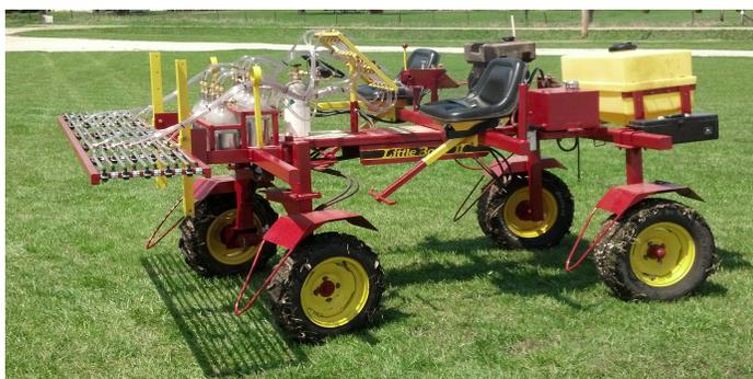
**Figure 2. Self-propelled research sprayer built by Iowa State personnel.**
