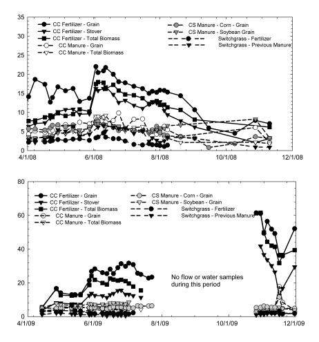
Figure 1. Flow-weighted nitrate-nitrogen concentrations in subsurface drainage water during 2008 and 2009 (note scale differences in 2008 and 2009).
