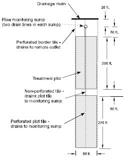
Figure 3. Example plot layout for two plots.
