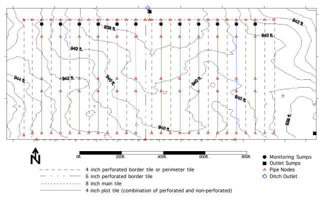
Figure 4. Drainage system layout.
