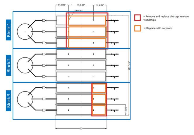
Figure 1. Schematic of the excavation and corn cob refill plan for the pilot-scale bioreactors. Block 2 was maintained as the woodchip filled control; block 1 was excavated to 3/4 the bioreactor length and refilled with corn cobs; block 3 was excavated to 1/4 bioreactor length and refilled with corn cobs.
