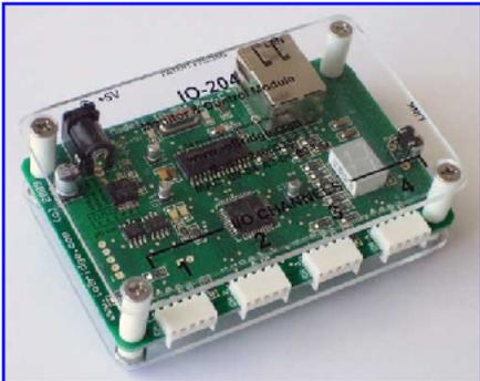
The IO-204 Monitor & Control Module is a green printed circuit board (PCB) housed in a white plastic enclosure. It features a central microcontroller, various integrated circuits, and several connectors. A USB Type-A port is visible on the right side, and a power jack is on the left. The board is populated with numerous surface-mount components and has a white label with the text 'IO-204 Monitor & Control Module'.
