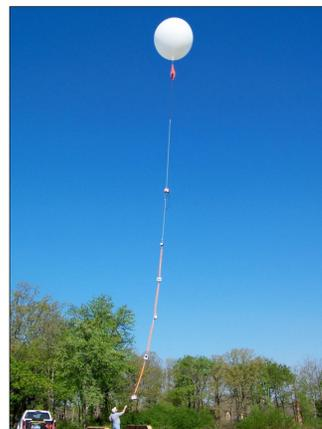
Figure 1: Inflated balloon with payload boxes before liftoff.
