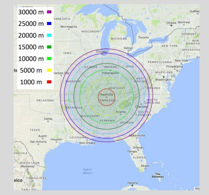
An amateur radio repeater was included in the balloon payload. The repeater was through to be a fun and engage tool to reach out to the surrounding community about the Eclipse Project. At altitude, the repeater would have a radio horizon sufficient to relay messages across the southeast. The furthest contact made during flights was in Cincinnati, OH.
