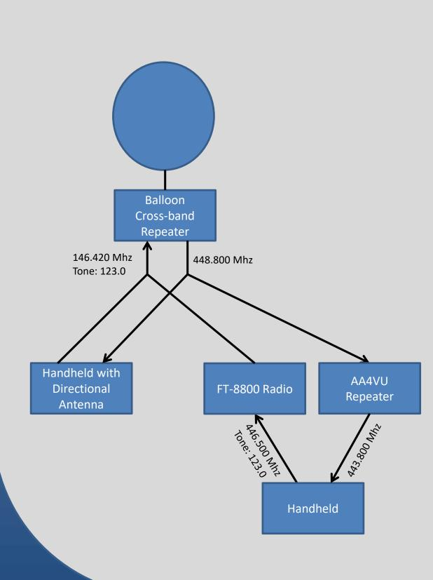
The balloon package operated as a cross band repeater. Any operator with a radio that could be programmed to operate in a cross band mode and an appropriate antenna could communicate through the repeater. In the Nashville area, a repeater relay was set up for better reception. Using the higher power and sensitivity of the repeaters to boost reception.
