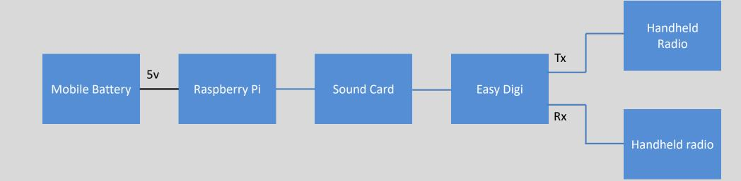
The repeater used a Raspberry Pi with the OpenRepeater package to manage transmission. Two Baofeng radios were used to receive and transmit.
