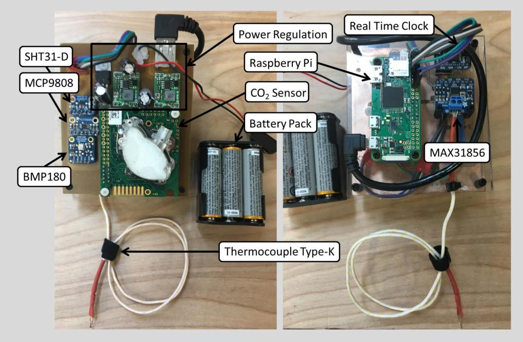
The environmental package utilized a Raspberry Pi Zero W to access and log the sensor data. The Pi ran a python script to iteratively access all the sensors on each of the digital buses.
