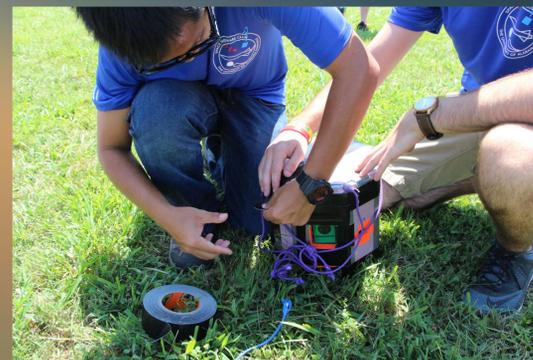
Preparing the line can be the most time consuming process during the ballooning process. Since line mass must be accounted for in the predictions, we cut our lines to length the day before a flight. Lines are secured to payloads by figure of eight knots for maximum strength and security. We also make sure that there is at least 15 ft. between parachute and the balloon to prevent parachute fouling.
