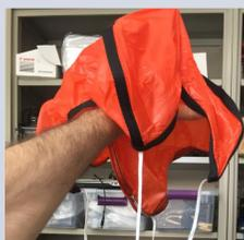
2-ft parachute worked well for 200 g payload
