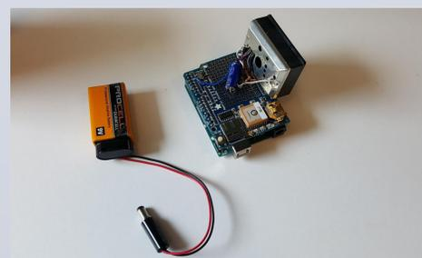
Dust sensor mounted on Arduino and GPS logger shield
