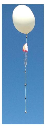
Fig. 3-4 Flight 282 at beginning of launch showing four PODS and the parachute with a enclosed 100g balloon. The internal probe boom is not visible but is located inside the balloon.
