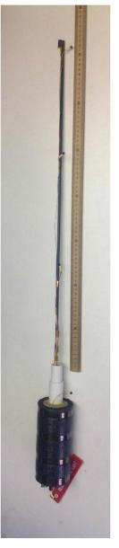
Fig. 3-2 internal temperature boom for insertion into nozzle.
