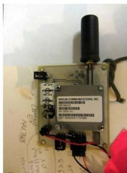
Photo 1. Iridium SBD9602 modem board with Sarantel helical antenna [www.elktronics.com](http://www.elktronics.com).
