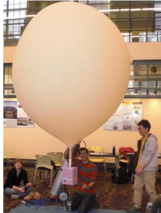
The Float payload during a venting test in which two pounds of excess lift were vented in under 5 minutes. The vent was successfully opened and closed by the DTMF/XBEE uplink. Vent status was monitored zigbee radio.
