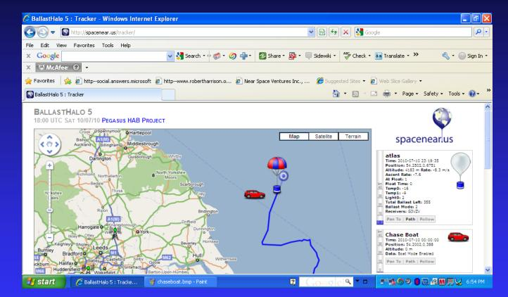
Telemetry must be uploaded in the following format: \$\$callsign, sequence, time(UTC), lat, lon, alt(m), sats, batt, temp\*<cksum>
