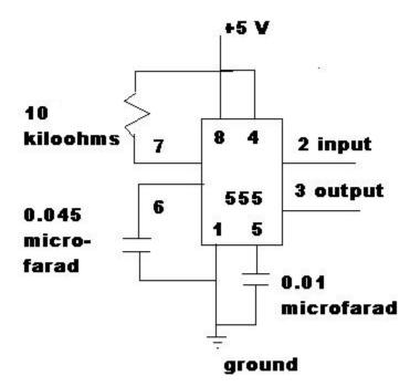
Figure 4. 555 One-Shot Timing Circuit Schematic diagram of 555 timing circuit. Input from Geiger counter goes into pin 2 and output to counting program comes out on pin 3. The RC time constant is determined by the resistor on pin 7 and the capacitor on pin 6.
