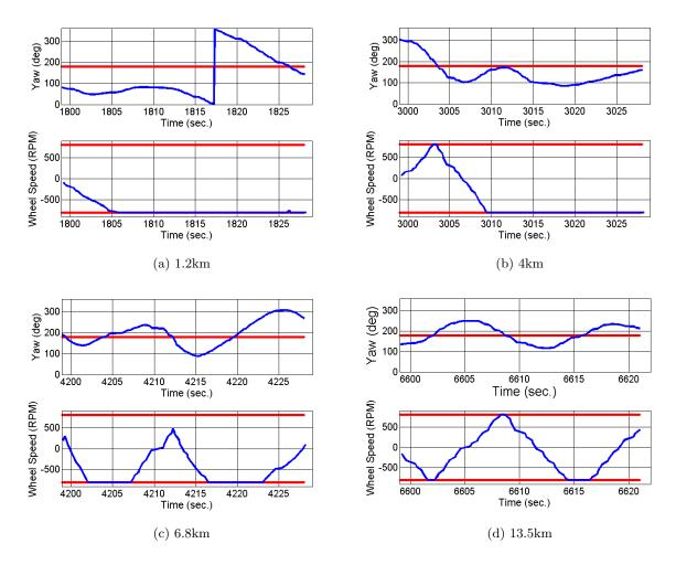
Figure 7: Platform yaw angle and motor RPM at various altitudes. Red line for yaw angle indicates the target pointing angle. Red lines for the motor RPM indicate saturation speeds.
