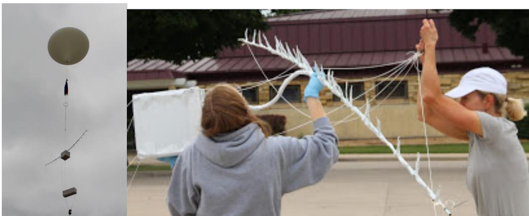
Fig. 4. The wake boom: Left side picture is a boom in flight and right is structure in preparation for flight. There is a 30 cm gap between the boom and the top of logging payload [22].
