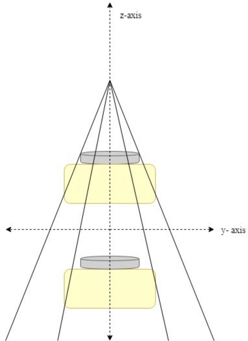
**Figure 8:** Vertical coincidence represented using two separated RM-80 Geigers.
