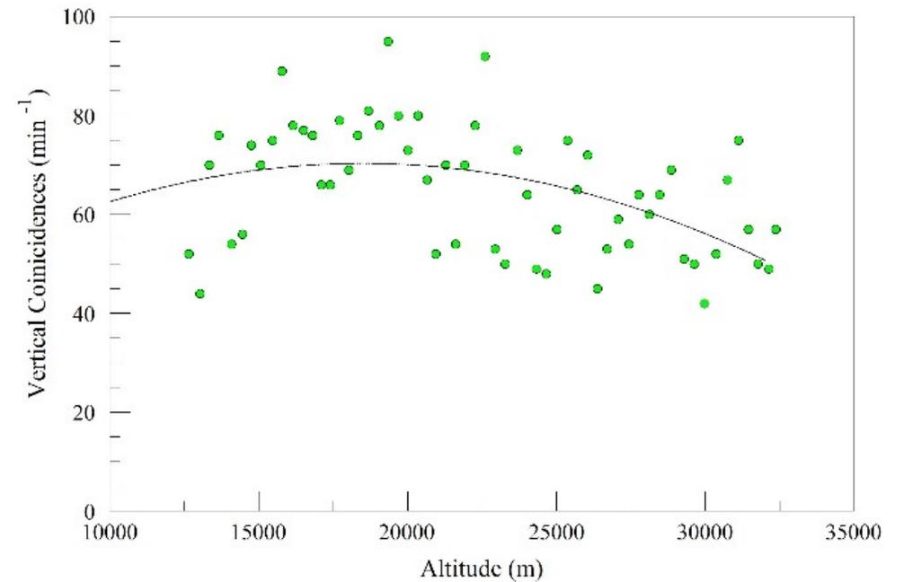
**Figure 21:** Plots of vertical and horizontal coincidence versus altitude on 6/13/19 flight.
