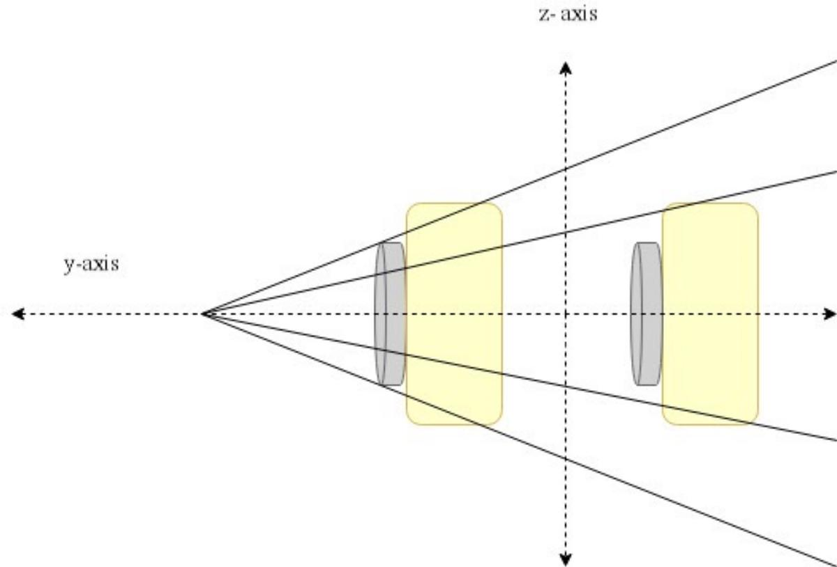
**Figure 9:** Horizontal coincidence represented using two separated RM-80 Geigers.
