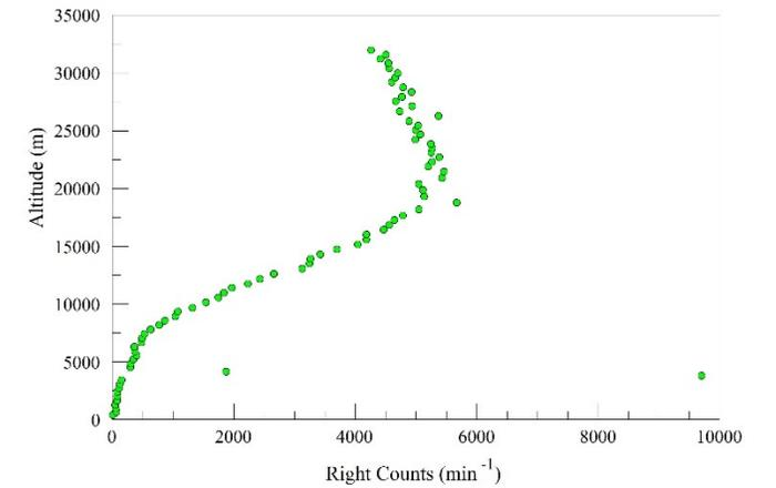
**Figure 16:** Total counts that were obtained from four RM-80 Geiger detectors on flight 6/7/19.
