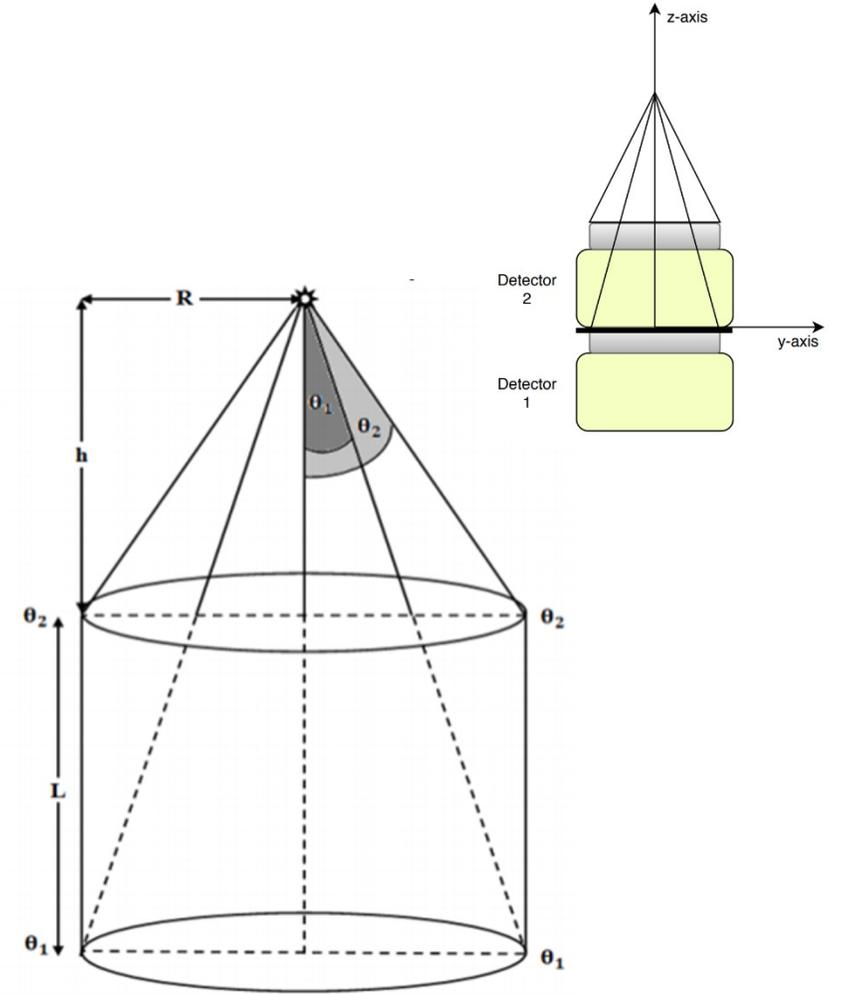
**Figure 7:** An axial point source with Cylindrical Detector.
