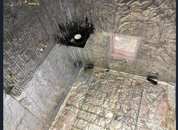
Cold Soak Box. Dry Ice was placed on the walls. A window allowed light in.
