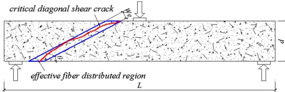
Figure 2. Effective fiber distributed region (EDR) in a beam
