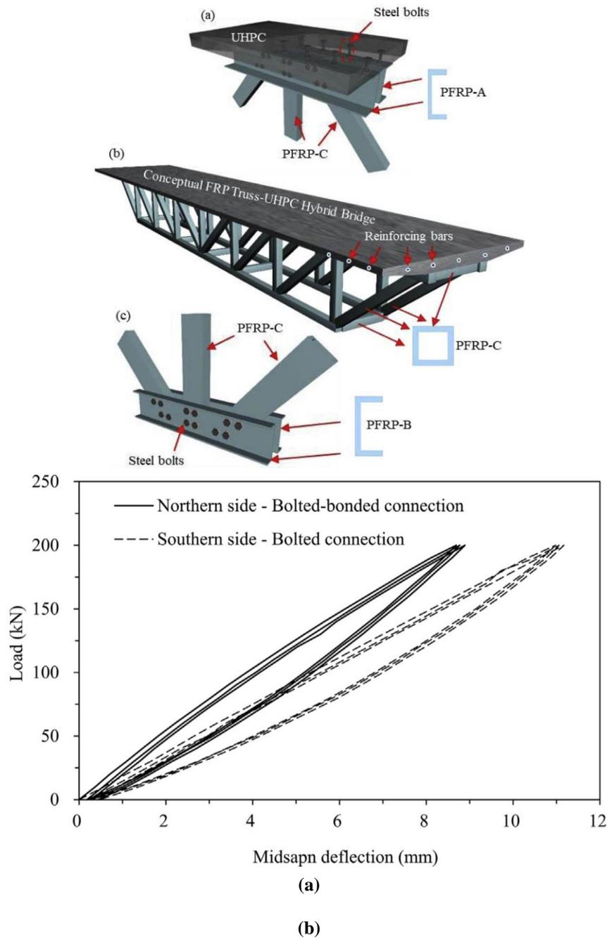
**Figure 4. (a) The proposed FRP truss-UHPC slab hybrid bridge, (b) load-deflection response of cyclic loading (Zou and Wang (2018)).**
