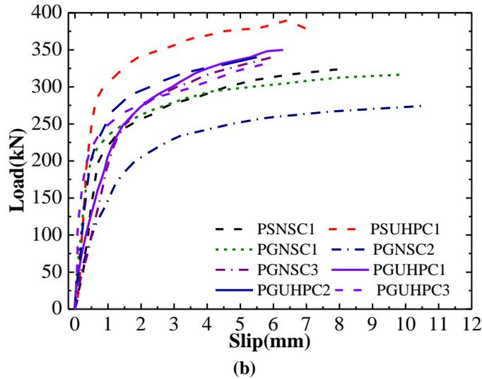
Figure 3. (a) Push-out test setup, (b) load-slip responses (Wang et al. 2018)
