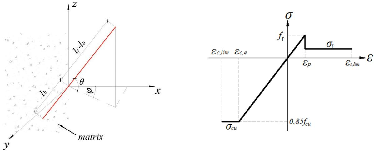
Figure 1. Ultra-high-performance fiber reinforced concrete constitutive model in compression and tension (Qi et al. 2018b)
