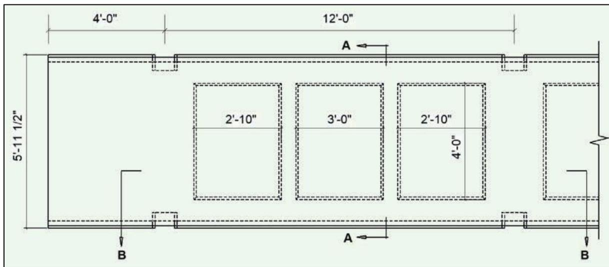
a) Plan view of the new precast concrete deck panel
