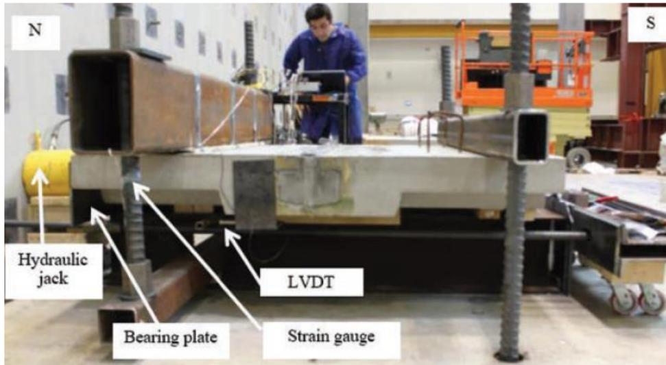
Figure 5: Push-off Test Setup for Steel Girder Specimens.
