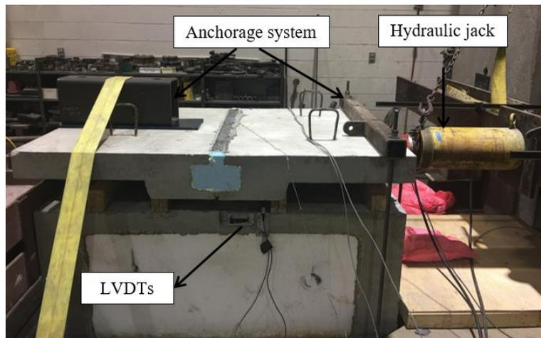
Figure 3: Push-off Test Setup for Concrete Girder Specimens
