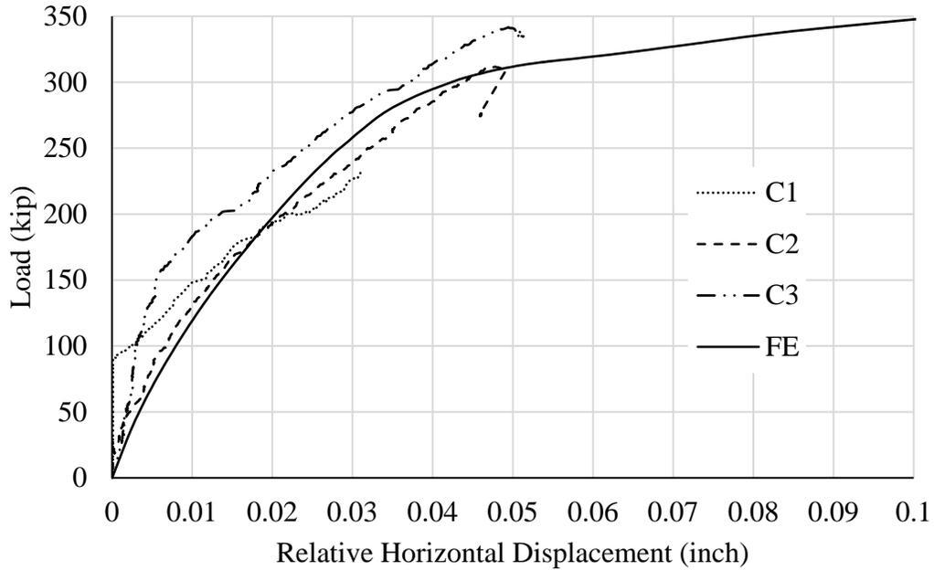
Figure 6. Load-displacement relationships of the three push-off specimens and FE model
