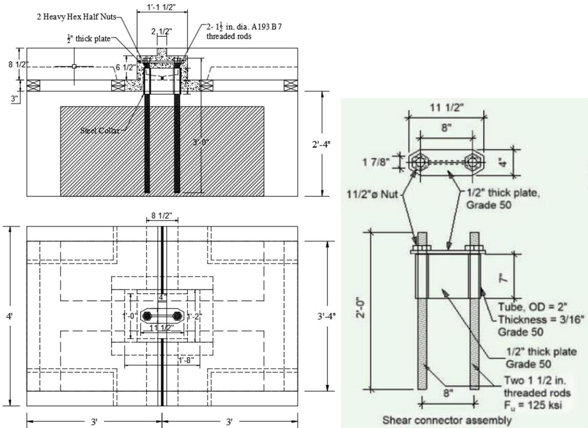
Figure 2: Push-off Test Specimen of UHPC Connection on Concrete Girder and The Connector Assembly (1in. = 2.54cm, 1ft = 0.3m).
