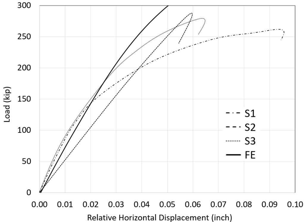
Figure 7. Load-displacement relationships of the three push-off specimens on steel girders
