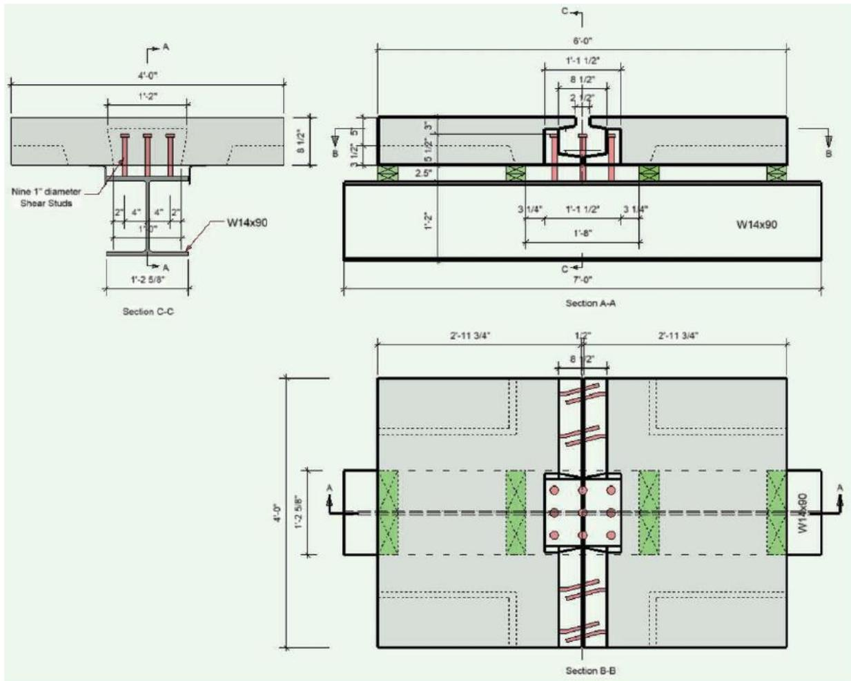
Figure 4: Push-off Test Specimen of UHPC Connection on Steel Girder (1in. = 2.54cm, 1ft = 0.3m).
