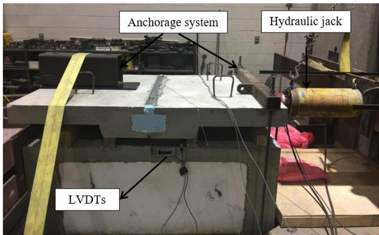
Figure 3: Push-off Test Setup for Concrete Girder Specimens
