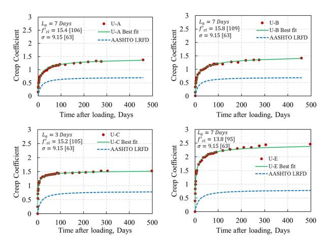
Figure 1. Creep coefficient of UHPC loaded at an early age
