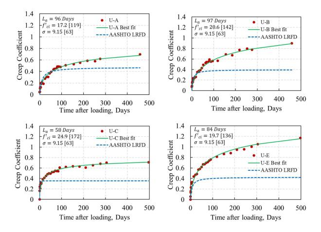
Figure 2. Creep coefficient of UHPC loaded at a mature age
