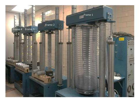
Figure 4. Creep cylinders in load frames
