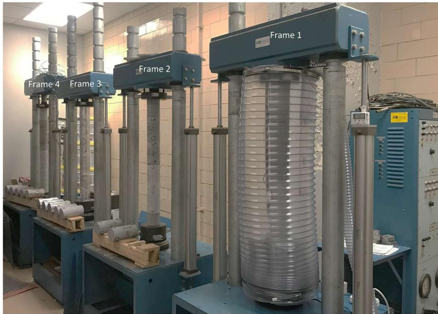
Figure 4. Creep cylinders in load frames
