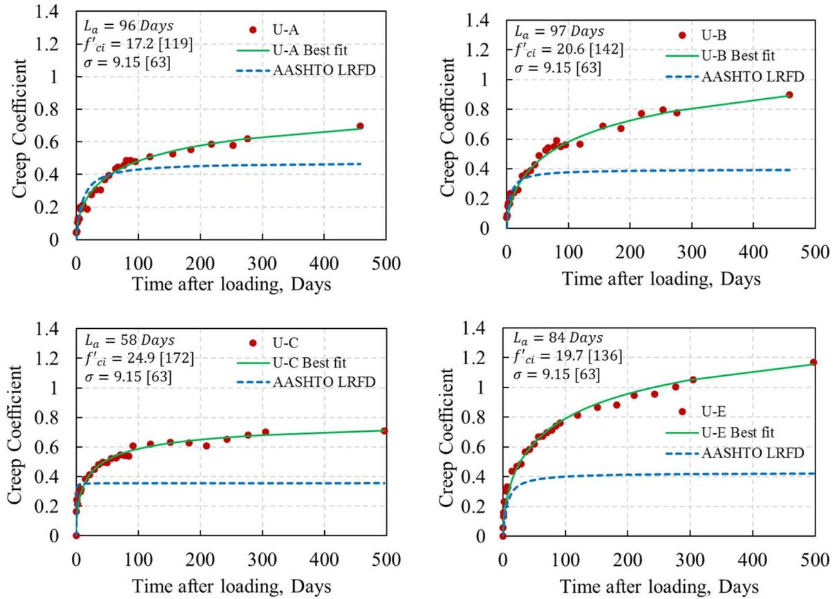
Figure 2. Creep coefficient of UHPC loaded at a mature age
