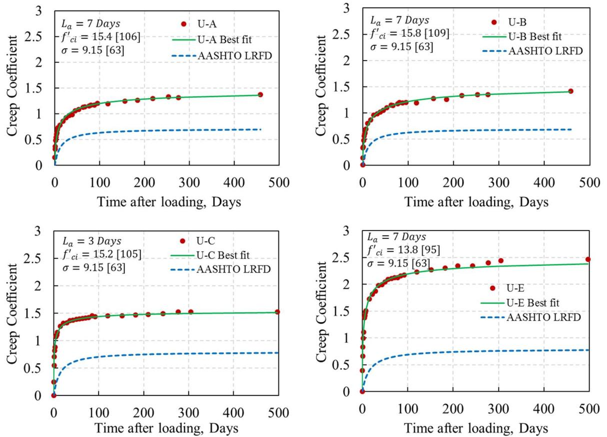
Figure 1. Creep coefficient of UHPC loaded at an early age
