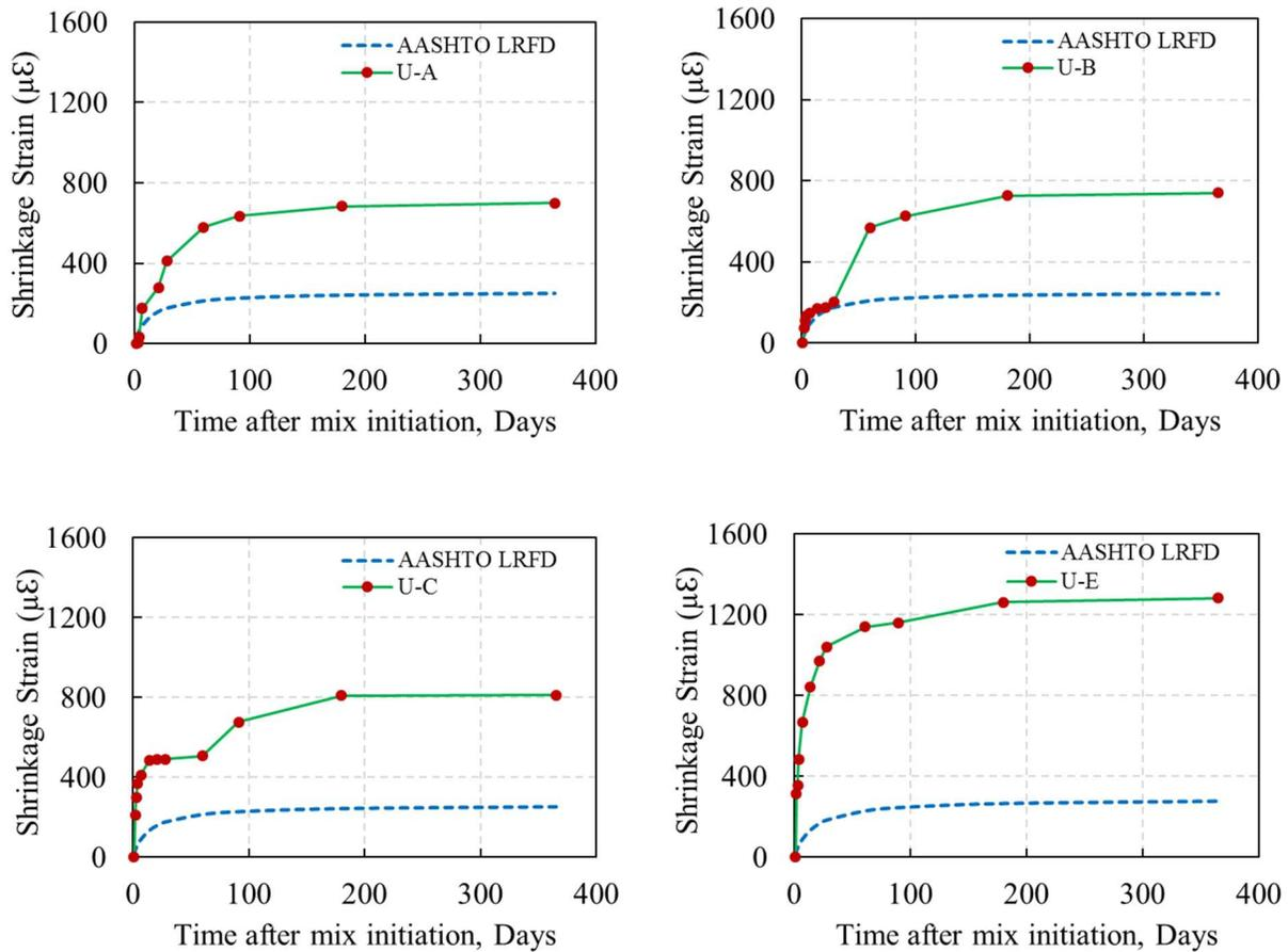
Figure 3. Strain due to total shrinkage of UHPC
