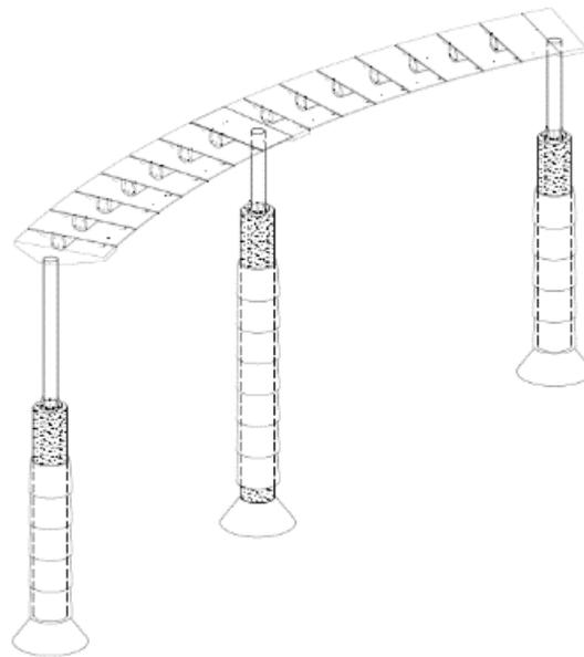
**Figure 5. Isometric view of UNAL footbridge.**
