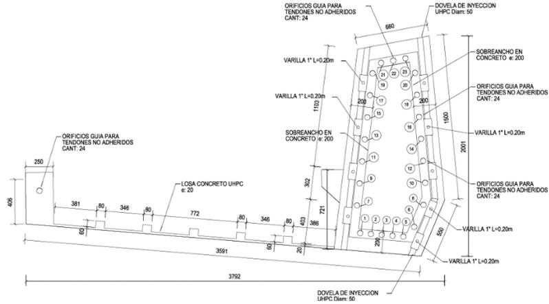
Figure 2. Cross section of the EAFIT girder box.
