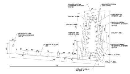
Figure 2. Cross section of the EAFIT girder box.
