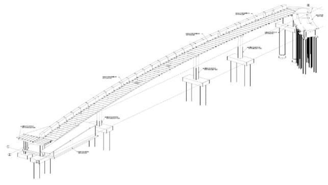
Figure 3.Isometrical view of EAFIT footbridge.
