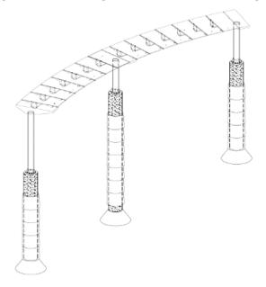
Figure 5. Isometric view of UNAL footbridge.
