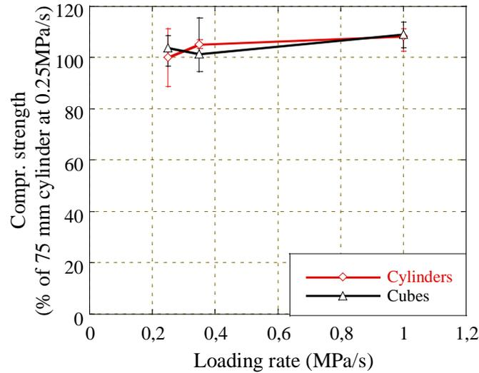
**Figure 2. Impact of specimen type and loading rate on compressive strength at mixing temperature of 20°C and curing temperature of 23°C**
