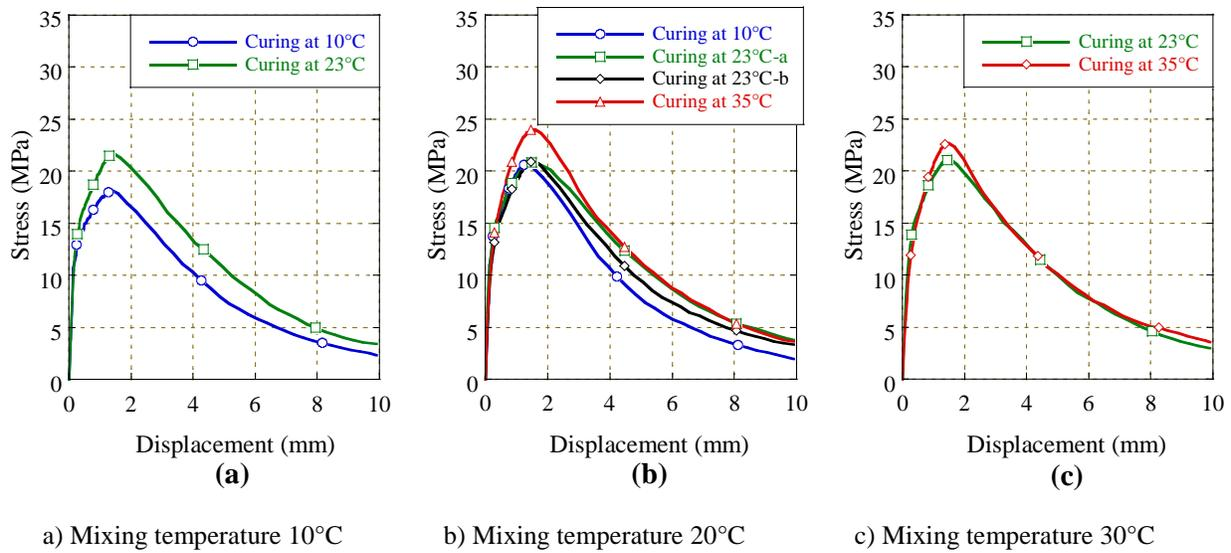
**Figure 3. Impact of curing temperatures on flexural strength**
