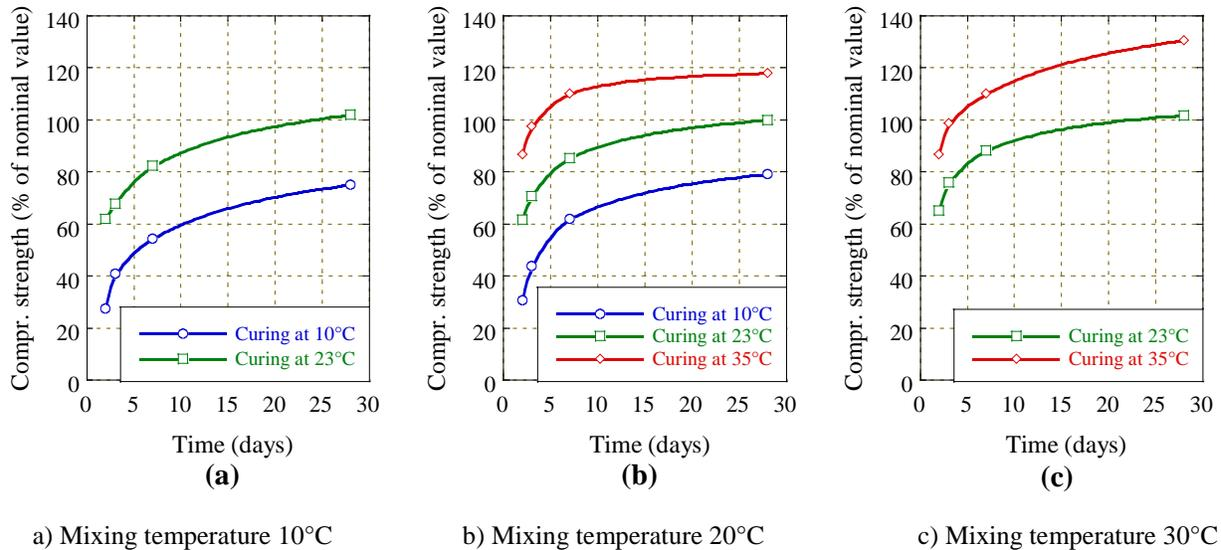
**Figure 1. Impact of curing temperatures on compressive strength**
