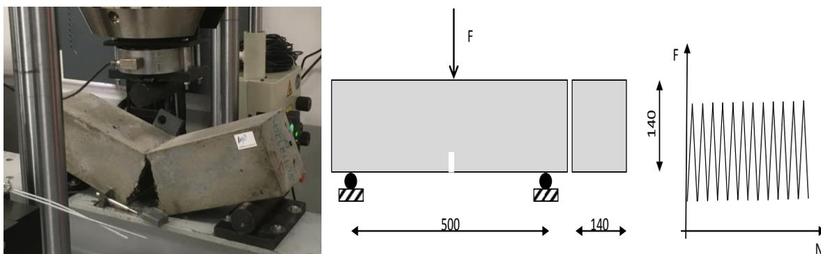
Figure 7. Fatigue test under UHPC
