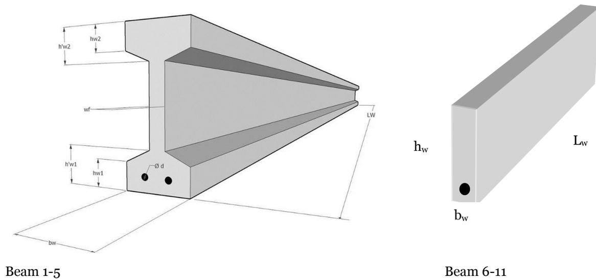
Figure 1. Geometrical parameters of beams
