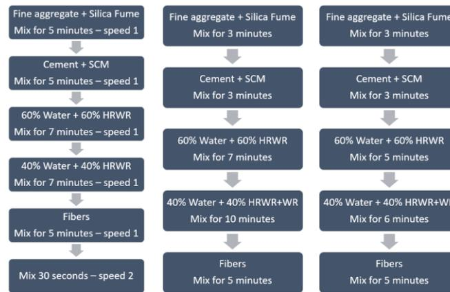
(a) Lab batch (b) Medium batch (c) Field batch
