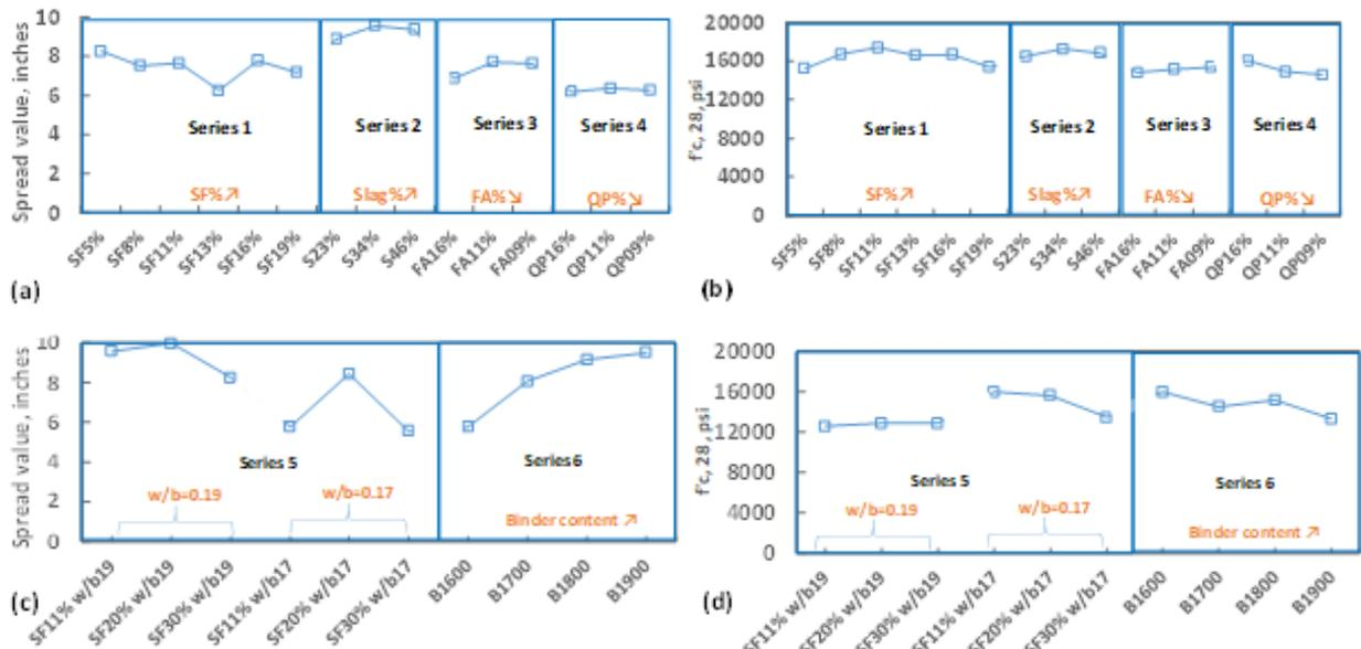
Figure 2. Impact of SCMs types and contents (a and b) and w/b and binder content (c and d) on fresh and hardened concrete properties (1 inch = 2.54cm; 1 psi = 0.0069 MPa)
