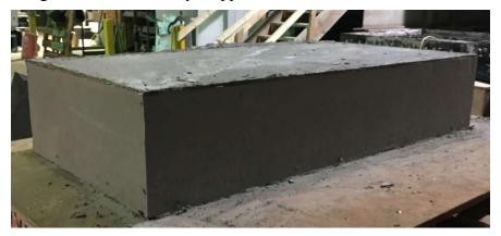
Figure 7 – UHPC Base Before Removing from Centre Forms
