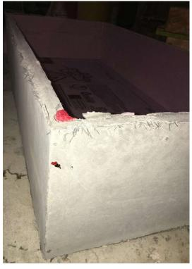
Figure 8 – Stripped UHPC Floating Base Prototype
