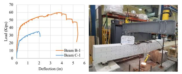
Figure 2: Load deflection plot and test setup
