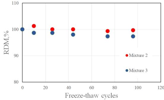
Figure 4 Effects of freeze-thaw cycling on RDM
