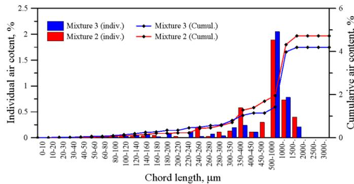
Figure 2 Air void size distribution based on the chord length from linear traverse method
