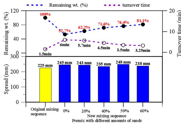
Figure 1 The weight variation of mixtures with different amounts of premixed silica sands
