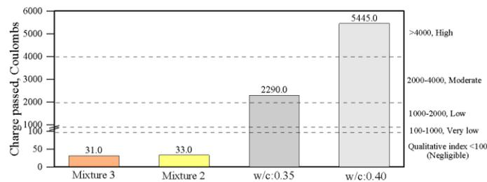
Figure 3 Total charge passed for UHPC and regular concrete
