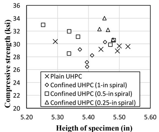
Figure 4. Compressive strength and height of cylinders.
