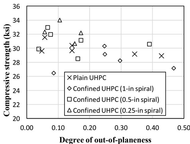
Figure 3. Compressive strength and cylinders end planeness of cylinders.
