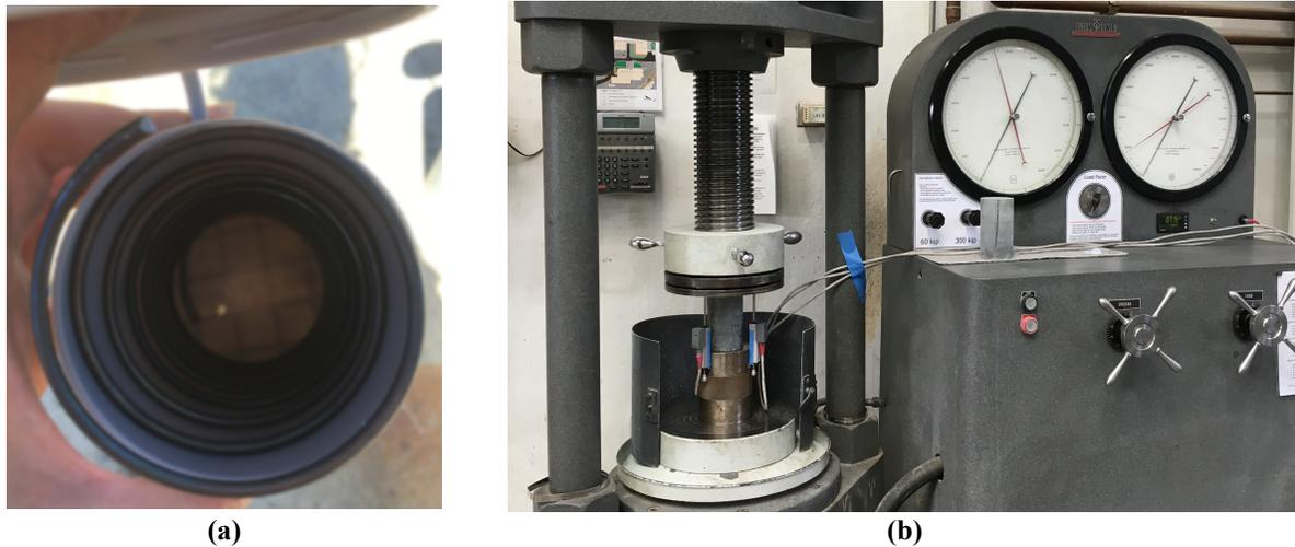
Figure 1. (a) Typical steel spiral inside the mold, (b) Tinius-Olsen testing machine and novotechniks arrangement (one is behind the specimen)
