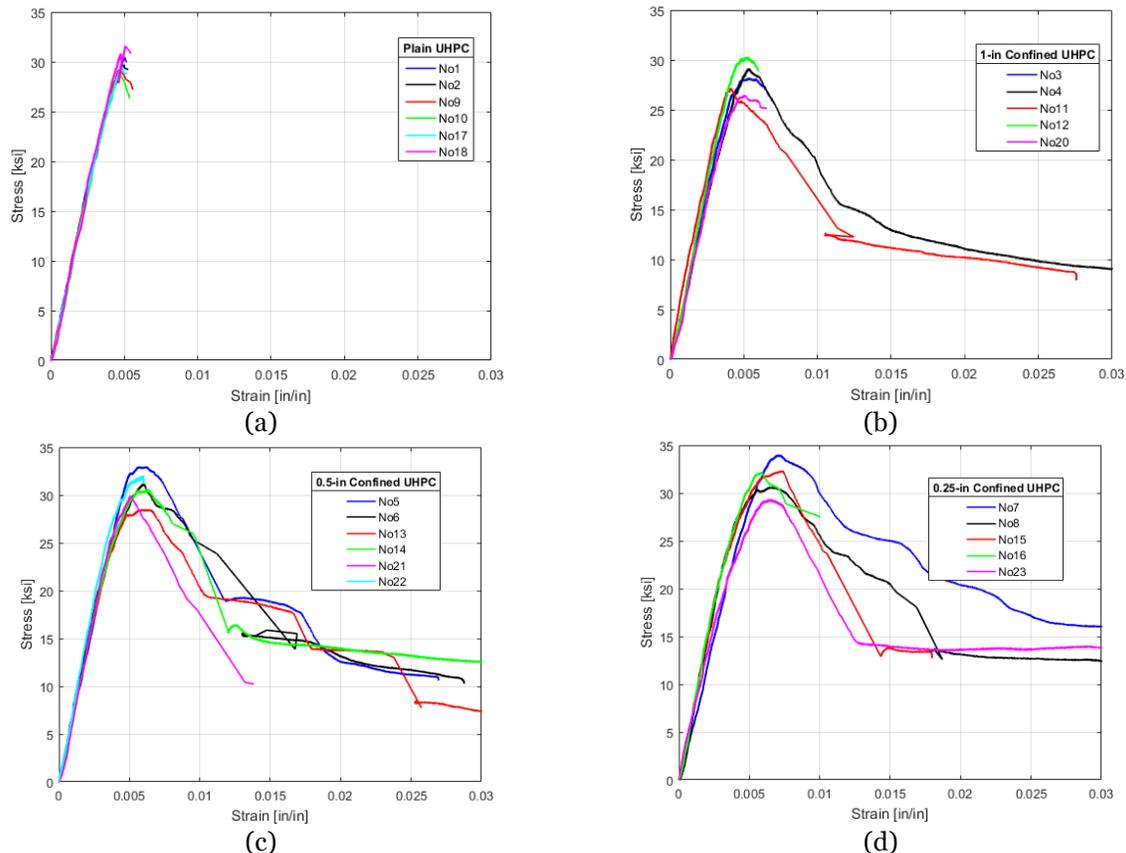
Figure 5. Stress-Strain response of (a) unconfined (plain) UHPC, (b) 1-in confined UHPC, (c) 0.5-in confined UHPC and (d) 0.25-in confined UHPC cylinders
