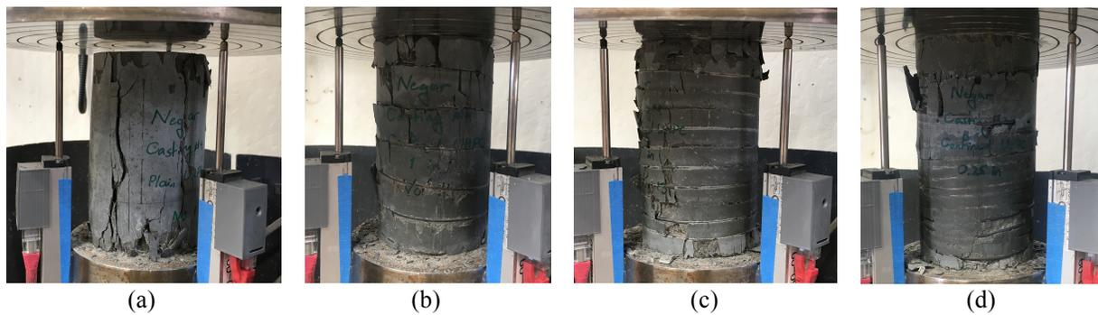
Figure 2. Typical failure mode of (a) unconfined (plain) UHPC, (b) 1-in confined UHPC, (c) 0.5-in confined UHPC and (d) 0.25-in confined UHPC cylinders
